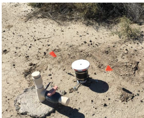
Figure 2-1 – Deployed Carbon Trap. NAVFAC EXWC ER-201582.
