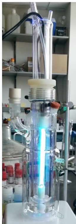
Figure 3.6. Photograph of photoreactor setup with 18 W UV LP Hg lamp.
