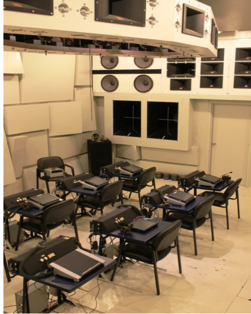
Figure 5. AFRL's VOCRES Facility used to Measure Speech Intelligibility Performance.
