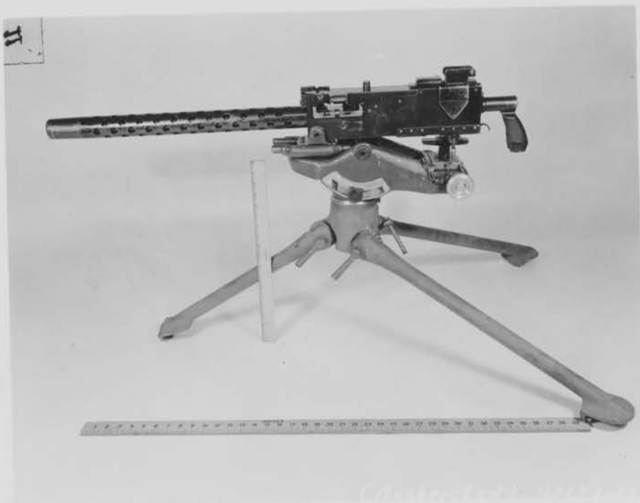
1919A4 Machine Gun, Cal. .30, mounted on T113 Tripod.
