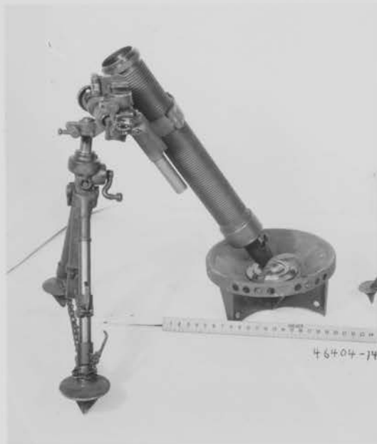
M21 Mortar with single section of firing tube and center section of base plate, for use as short barrel weapon.
