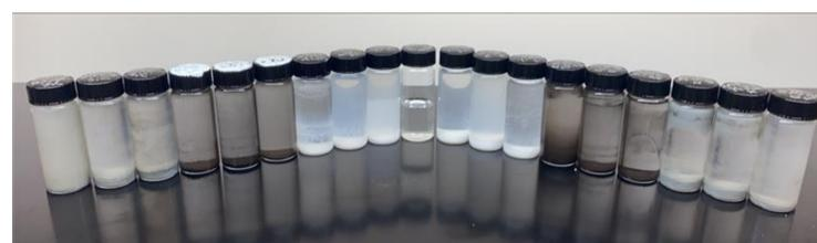
Figure 3. PSF-20cSt plus percentage variation of Alumina, Silicon Carbide and Iron (II,III) Oxide with and without surfactants
