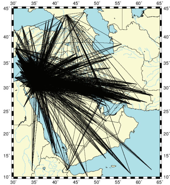
Figure 19. Ray path coverage of the seismic events recorded by the JSO network shown in Figure 18.
