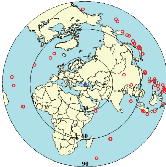
Figure 38. Teleseismic events (red circles) recorded at station KIV (blue triangle) are utilized for receiver function analysis for the station. The three black circles indicate epicentral distances of 30, 60 and 90 degrees, respectively.
