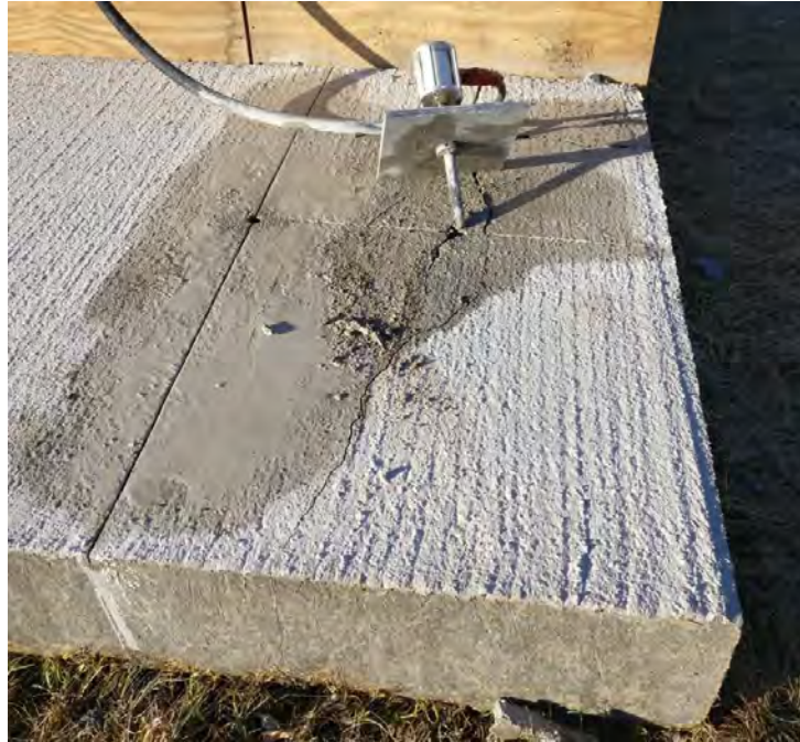
Figure 128. Shot 10: Large Cracks Did Not Follow Pre-cut Lines.
