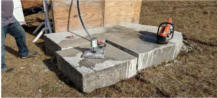
Figure 149. Shot 14: Plasma Blasting Probe in Concrete Section Separated by Shot 13
