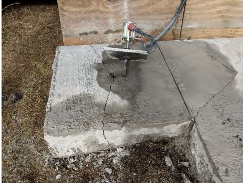
Figure 161. Shot 16: Plasma Blasting Probe Failed; Cracks Did Not Follow Pre-cut Line
