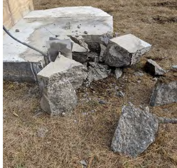
Figure 153. Shot 14: Debris And Concrete Chunks from Separated Concrete Section
