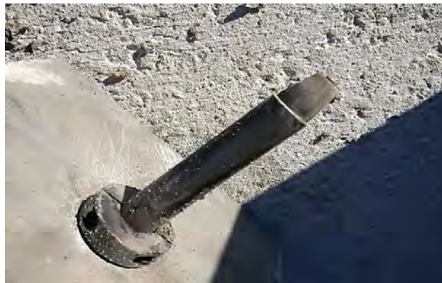
Figure 87. Plasma Blasting Test Probe after Shot 3
