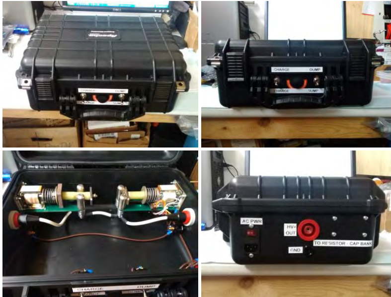
Figure 35. Constructed Field-portable HV Charge/Dump Control Switches
