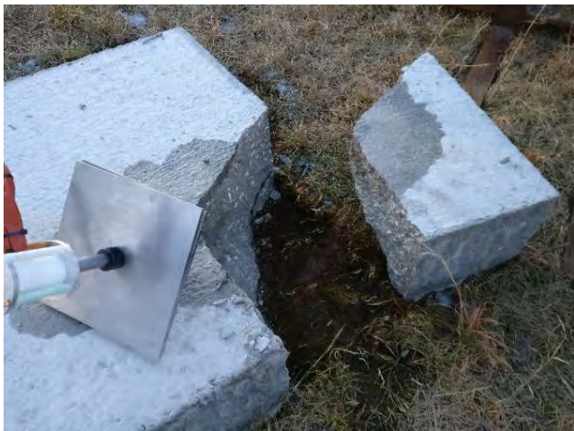
Figure 78. Shot 2: Fractured Section after Separated Concrete Section Pulled Back
