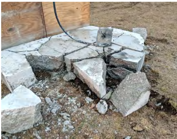
Figure 184. Shot 20: Debris and Chunks from 36-in by 36-in Shot 19 Fragment
