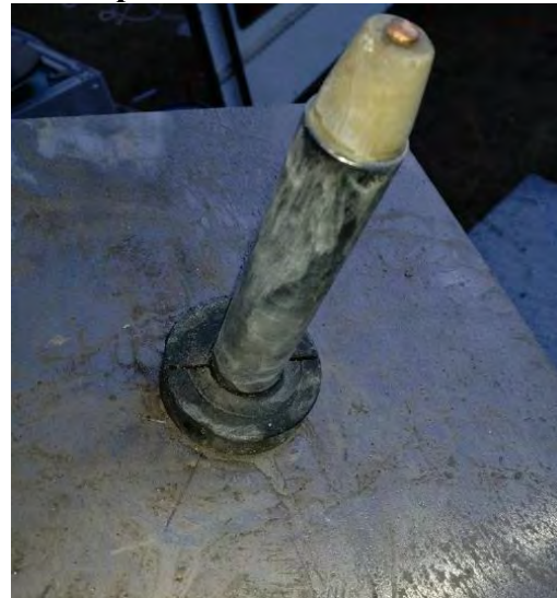
Figure 81. Photo of Plasma Blasting Test Probe after Shot 2; No Damage Noted to Probe
