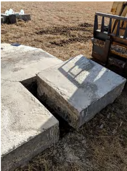
Figure 147. Shot 13: Separated Section of Concrete with Crack
