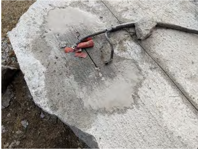
Figure 173. Shot 18: Pressure Pulse of Exploding Wire Only Lifted Concrete Chunk
