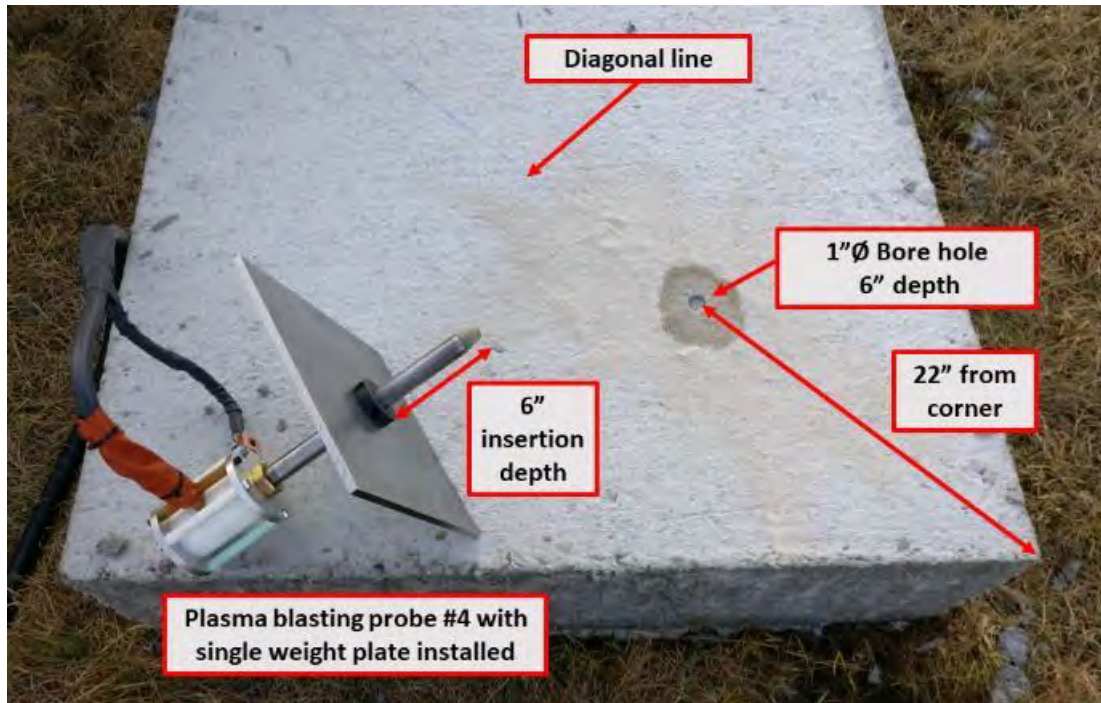
Figure 70. Shot 1: Concrete Test Slab and Plasma Blasting Probe Setup Table 7. Data for Shot 1: Test Setup and Results
