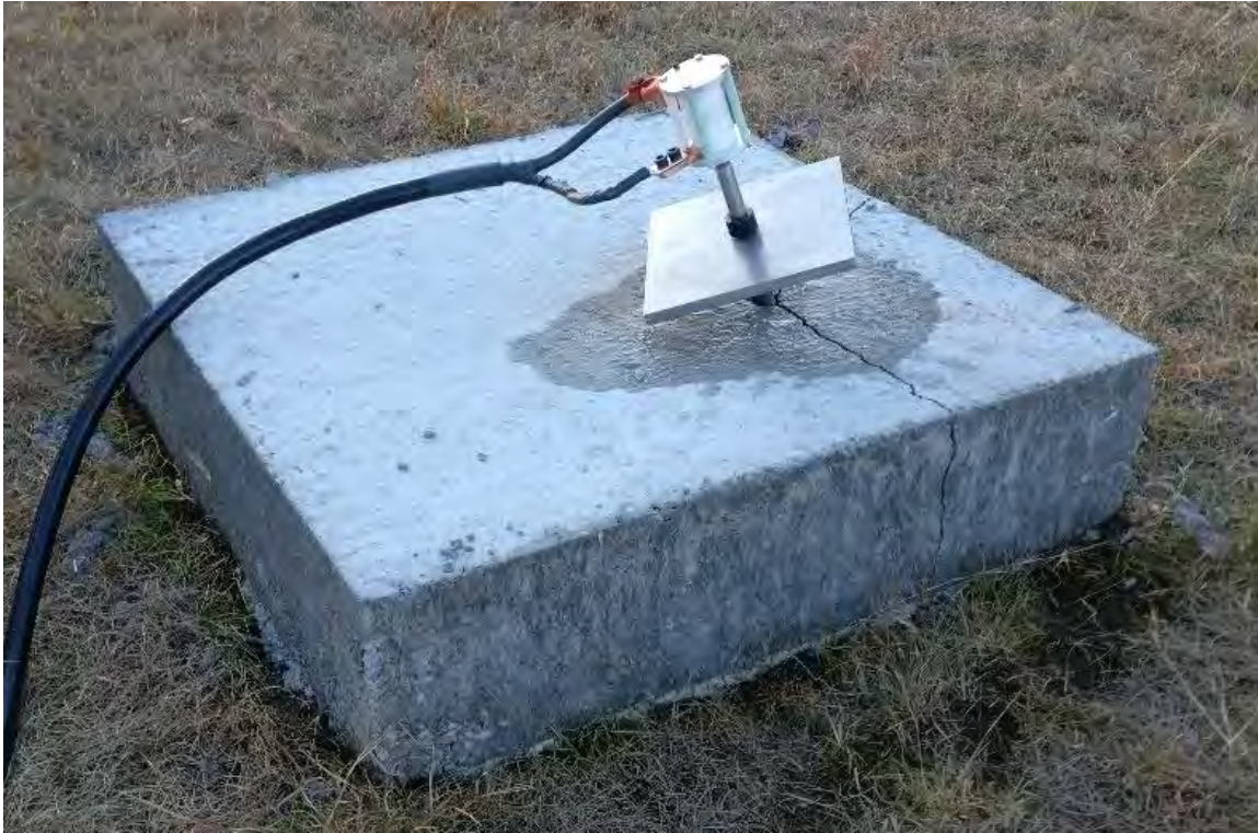
Figure 76. Shot 2: Concrete Test Slab Successfully Fractured
