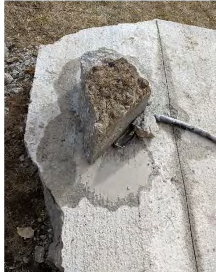
Figure 170. Shot 19: Chunk of Concrete over Wire and Cut to Contain Pressure Pulse
