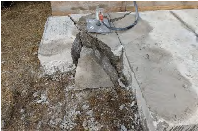
Figure 166. Shot 17. Crack Propagation Did Not Follow Offset Pre-cut Lines
