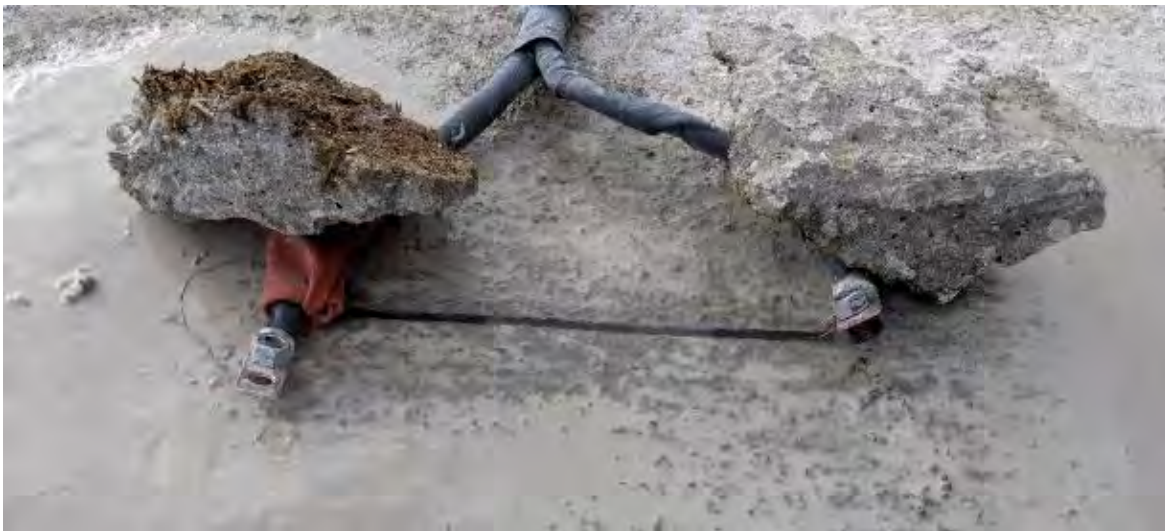
Figure 168. Shot 18: Exploding Wire for Installation in Cut in Slab
