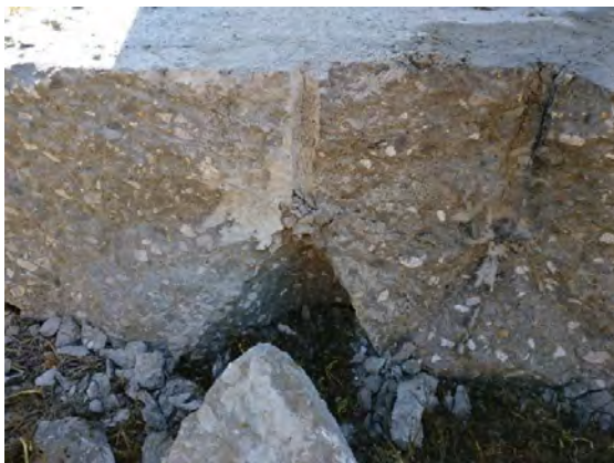
Figure 99. Shot 5: Conical Section Separated below Borehole
