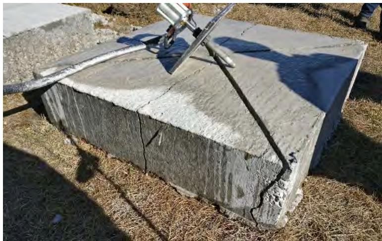
Figure 112. Shot 7: Corner Crack along the 2-in-deep Pre-cut Lines in Test Slab 3
