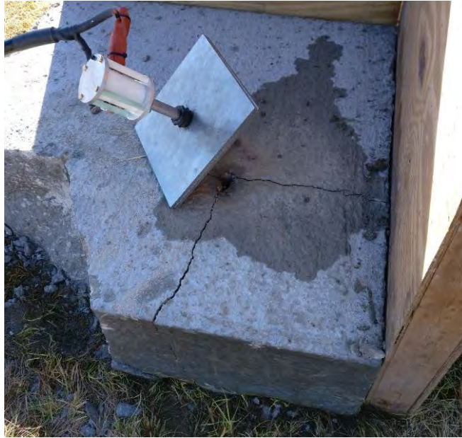
Figure 91. Shot 4: Separated Corner of Test Slab; Repeats Shot 2 Result
