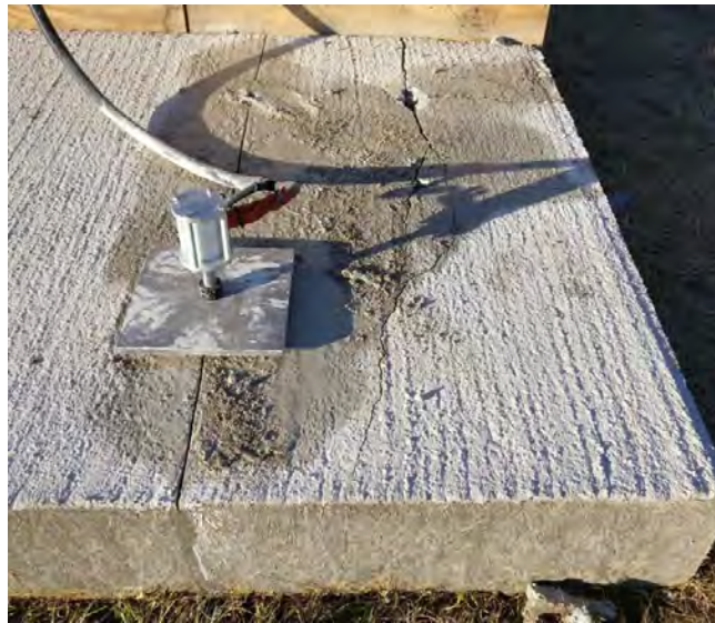
Figure 129. Shot 11: Placement of Plasma Blasting Probe in Borehole
