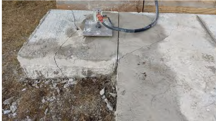
Figure 163. Shot 17: Probe in Hole between Hole for Shots 15 & 16, and Cut in Test Slab 4
