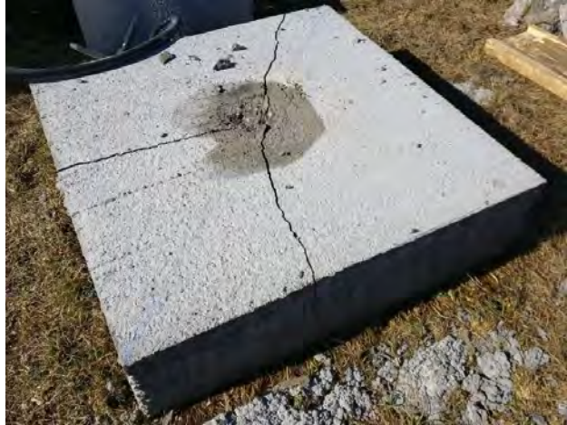
Figure 104. Shot 6: Concrete Test Slab Cracked into Three Sections
