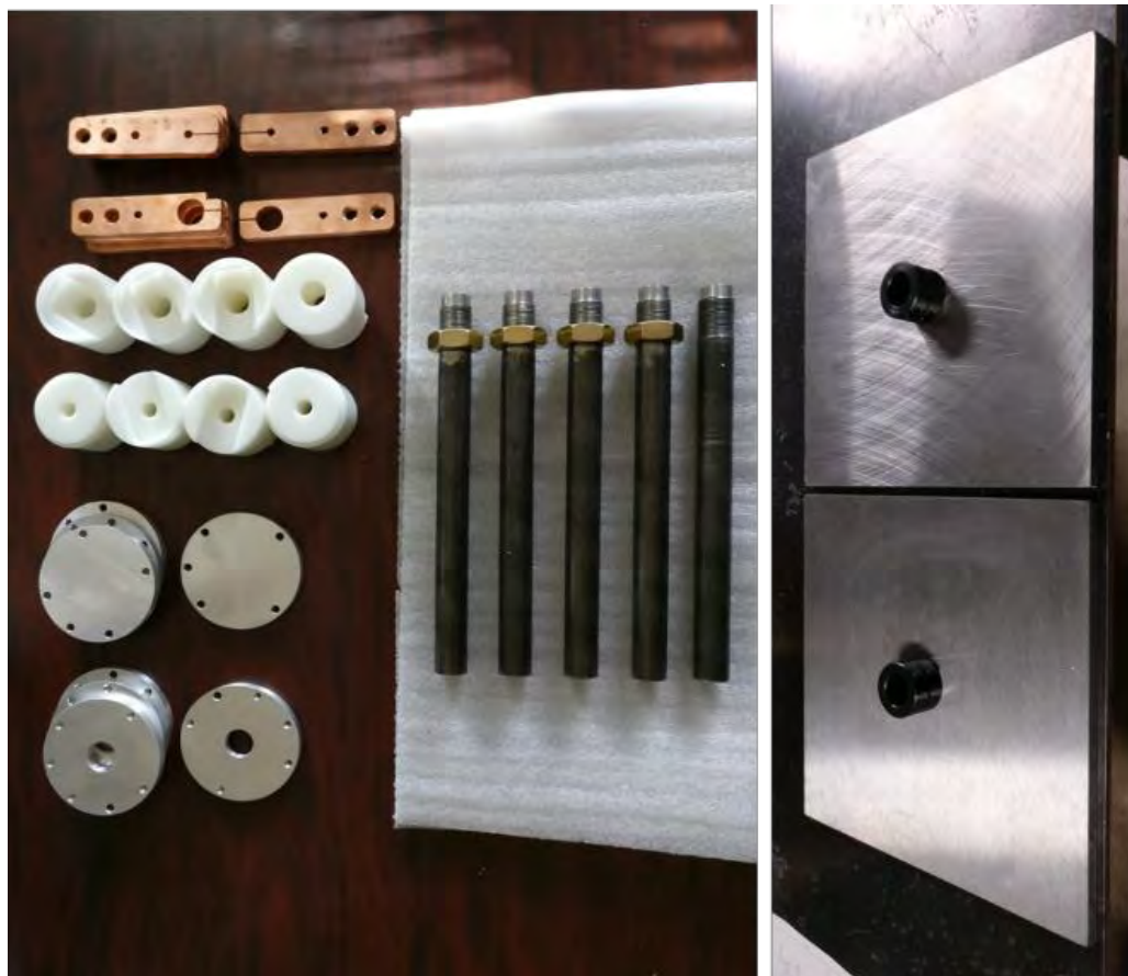
Figure 26. Machined EHF Plasma Probe Parts (left) and Inertial Blast Restraint Plates (right)
