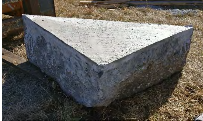
Figure 114. Shot 7: Crack Cross-section of Chunk Separated along Pre-cut Diagonal Lines
