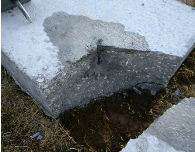
Figure 78. Shot 2: Fractured Section after Separated Concrete Section Pulled Back
