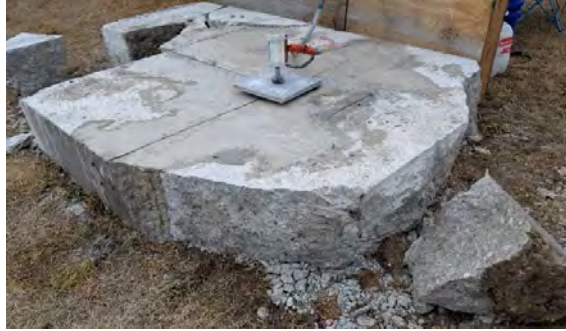
Figure 175. Shot 19: Test Setup with Plasma Blasting Probe Installed
