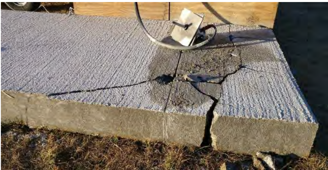
Figure 132. Shot 11: Cracks and Chunk Separation from Concrete Test Slab
