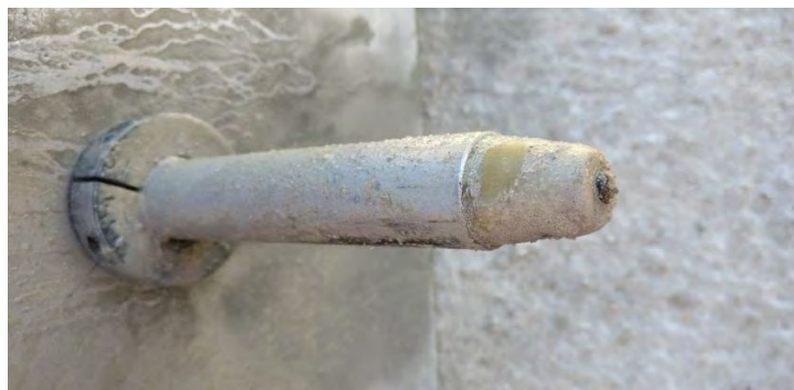
Figure 93. Plasma Blasting Test Probe after Shot 4
