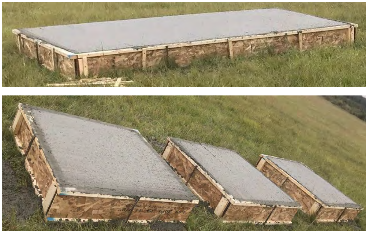
Figure 36. 12-in-thick Concrete Pads for EHF Testing: (top) 6-ft x 12-ft Slab, (bottom) Three 6-ft x 6-ft Slabs
