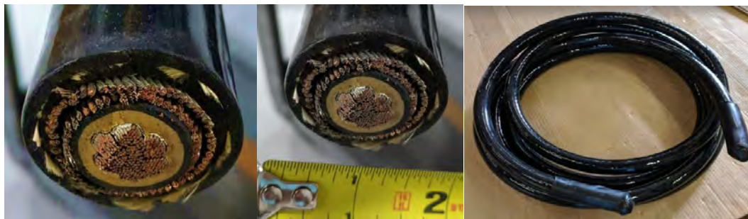
Figure 28. EHF Pulse Transmission Line, Dielectric Sciences 2198 Coaxial Cable Cross-Section and Overall Coil
