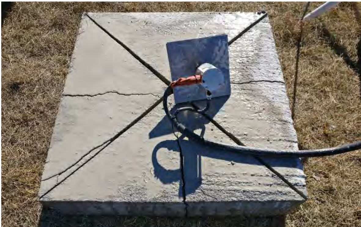
Figure 110. Shot 7: Crack Separation along the Pre-cuts of Test Slab 3
