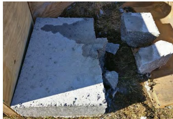
Figure 98. Shot 5: Remaining Section of Concrete Test Slab 1 after Debris Removal
