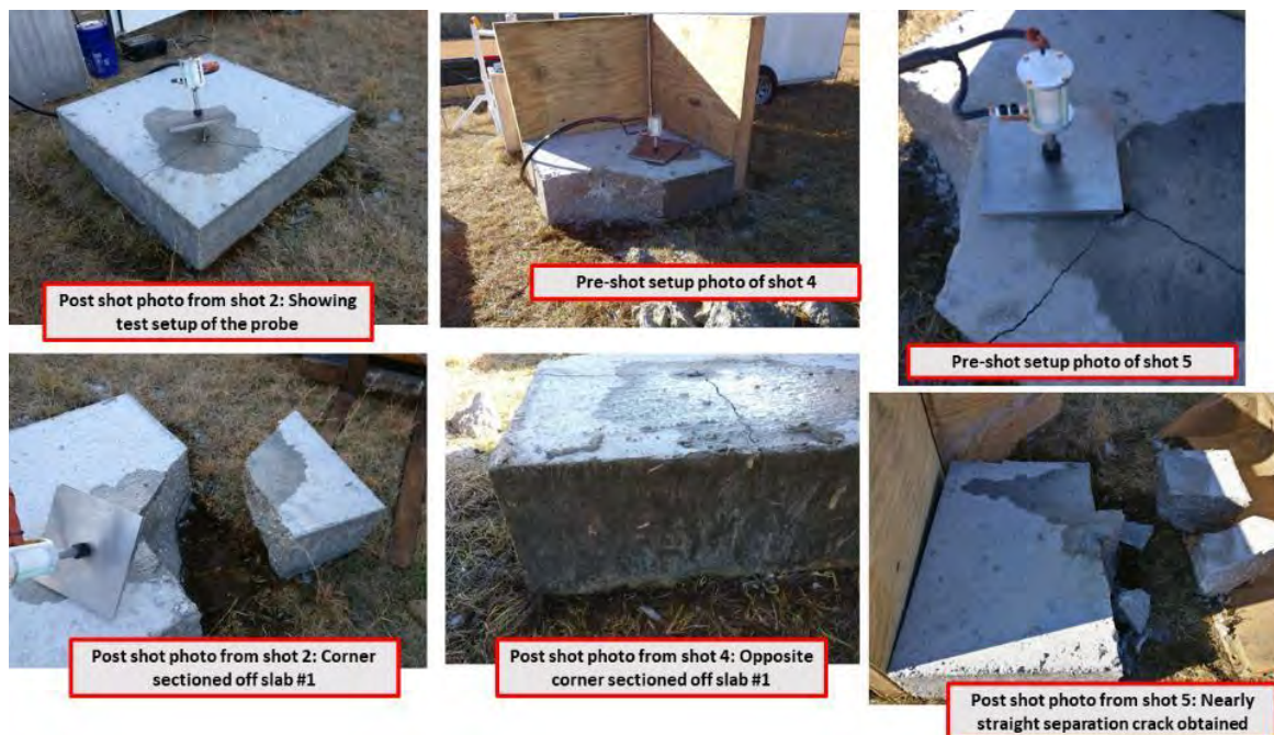
Figure 43. Sequence of Three Shots: (left) 2 Broke off a Section of Test Slab 1, (center) 4 Cracked along the Same Line; 5 (right) Left a Reasonably Straight Edge
