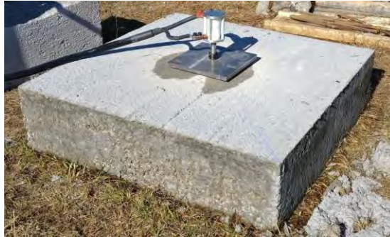
Figure 101. Shot 6: Setup; Borehole Drilled in Center of 4-ft x 4-ft Concrete Test Slab 2
