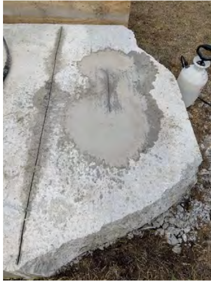
Figure 169. Shot 18:~ Cut into Concrete Test Slab 13 to Hold Exploding Wire
