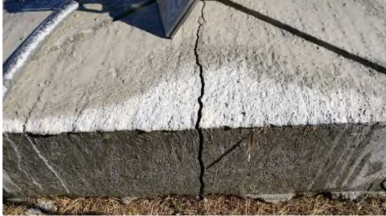
Figure 111. Shot 7: Close-up of an Unintended Transverse Crack in Test Slab 3
