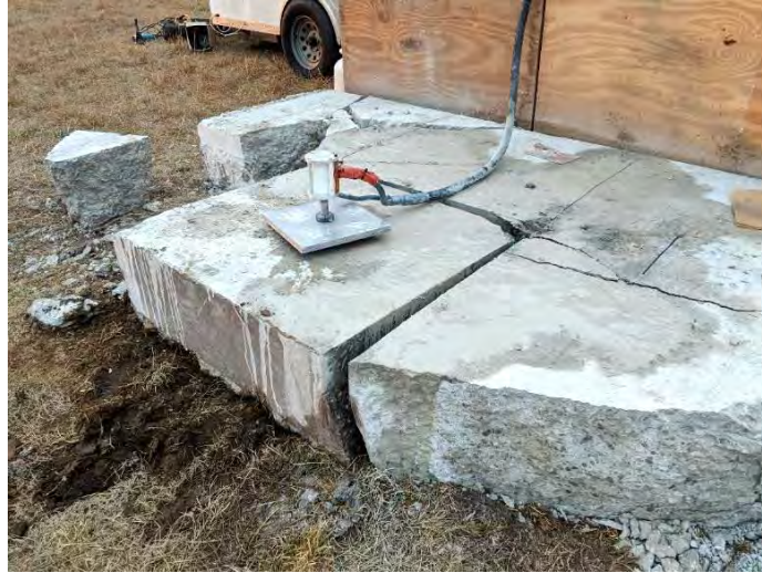
Figure 181. Shot 20: Plasma Blasting Probe in Concrete Section Separated by Shot 19
