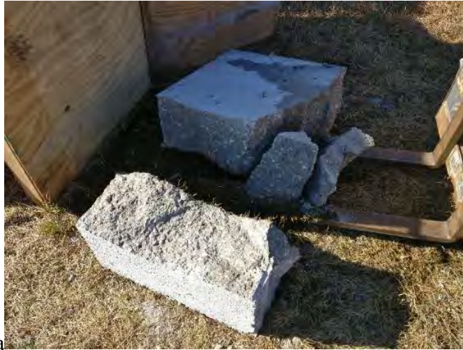
Figure 44. Remaining Section of Test Slab 1 Split into Two Pieces by Shot 5
