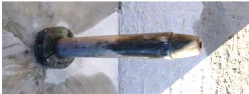
Figure 124. Plasma Blasting Test Probe after Shot 9
