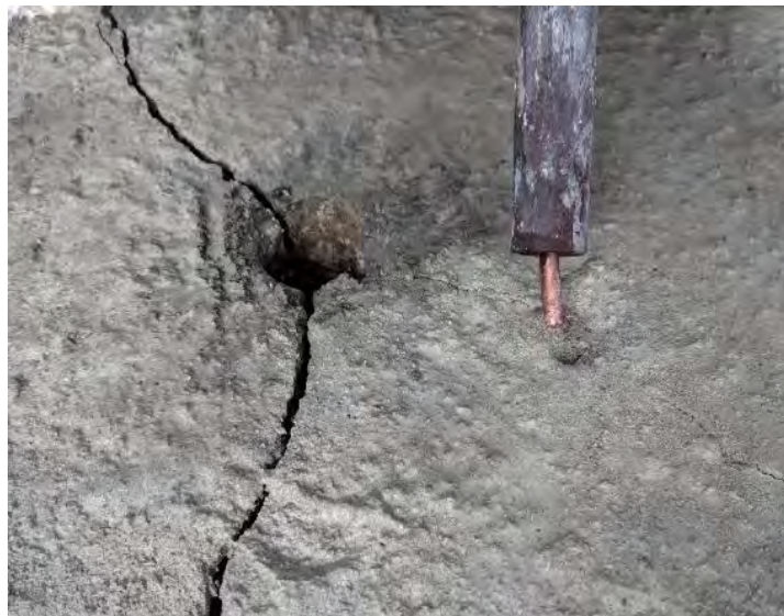
Figure 162. Shot 16: Failed Plasma Blasting Probe Tip and Cracks Formed from Borehole
