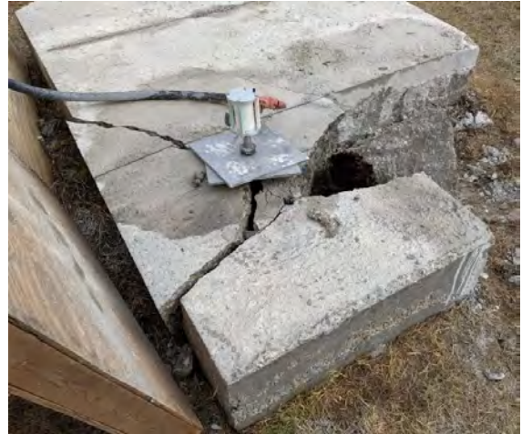
Figure 167. Shot 17. Crack Propagation Did Not Follow Offset Pre-Cut Lines
