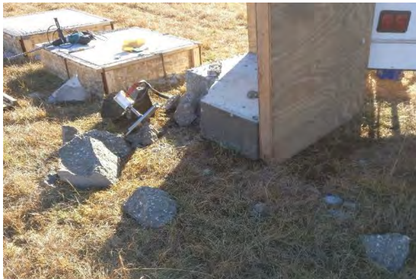
Figure 86. Shot 3: Debris; Fragments of Chunk of Concrete Separated by Shot 2
