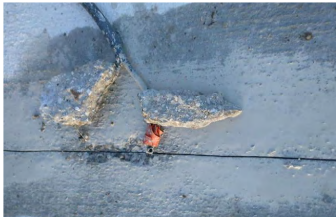
Figure 140. Shot 12: Exploding Wire Blasted out Shallow Divot along Wire in Pre-cut Line
