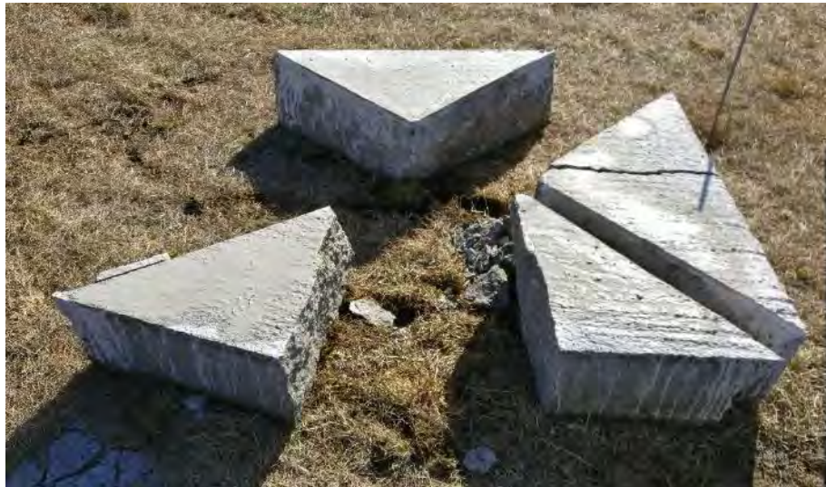
Figure 115. Shot 7: Unintended Cracks in Two Other Chunks Separated along Pre-cuts
