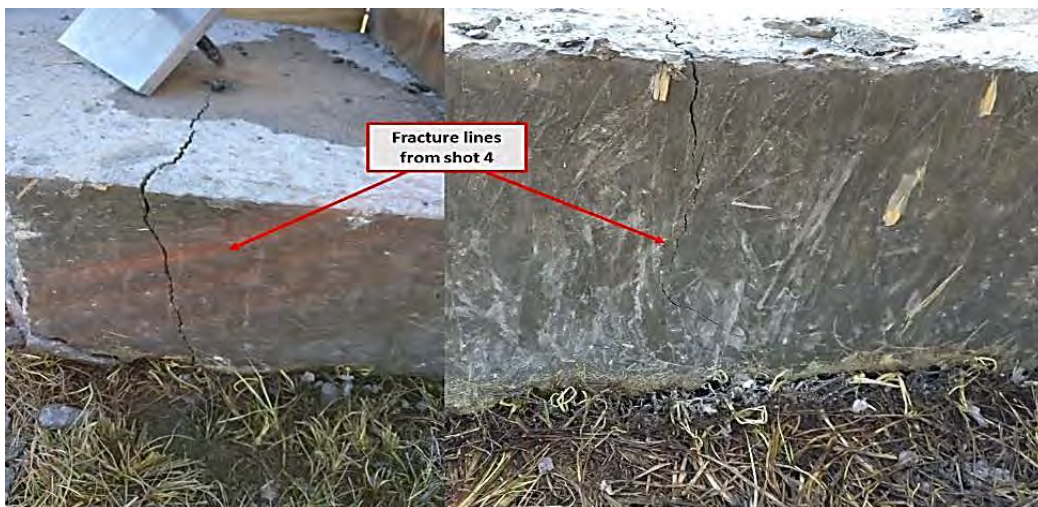
Figure 92. Shot 4: Fracture Lines in Concrete Test Slab 1
