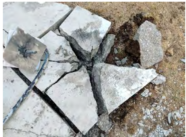
Figure 185. Shot 20: Debris and Chunks from 36-in by 36-in Shot 19 Fragment
