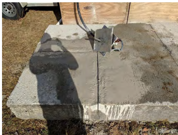
Figure 145. Shot 13: Cracked along Both Pre-cut Lines on 4 Concrete Test Slab
