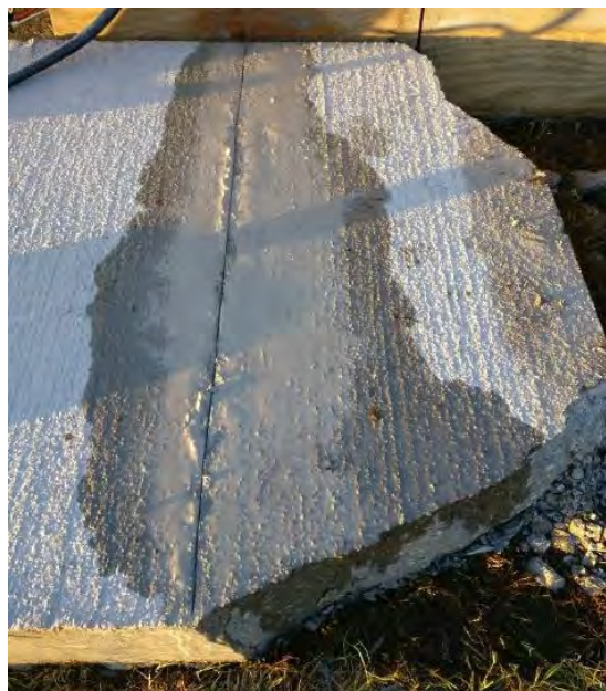
Figure 136. Shot 12: 2-in-deep Pre-cut Line for Exploding Wire Test
