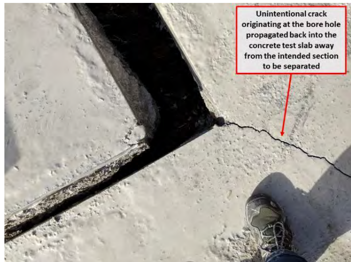
Figure 148. Shot 13: Unintentional Crack from Borehole into Concrete Test Slab
