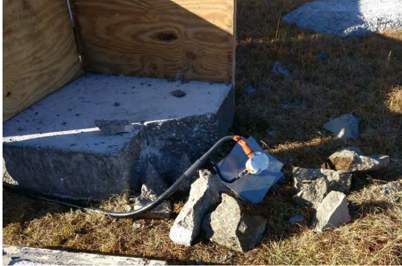
Figure 85. Shot 3: Completely Fractured Debris from Chunk of Concrete from Shot 2
