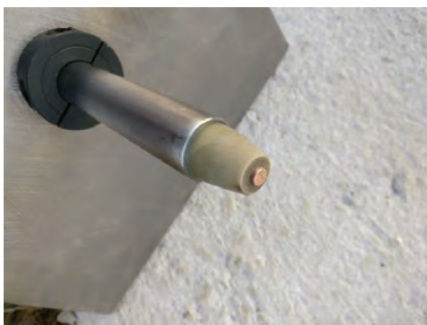
Figure 73. Plasma Blasting Probe Tip post Fire on Shot 1 (after Clean-up); No Visible Damage to Probe from the Shot
