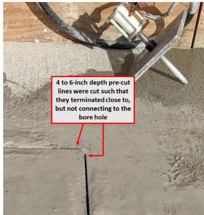
Figure 141. Shot 13: Pre-cut Lines End Close to (~0.5 in), but Do Not Connect to Borehole
