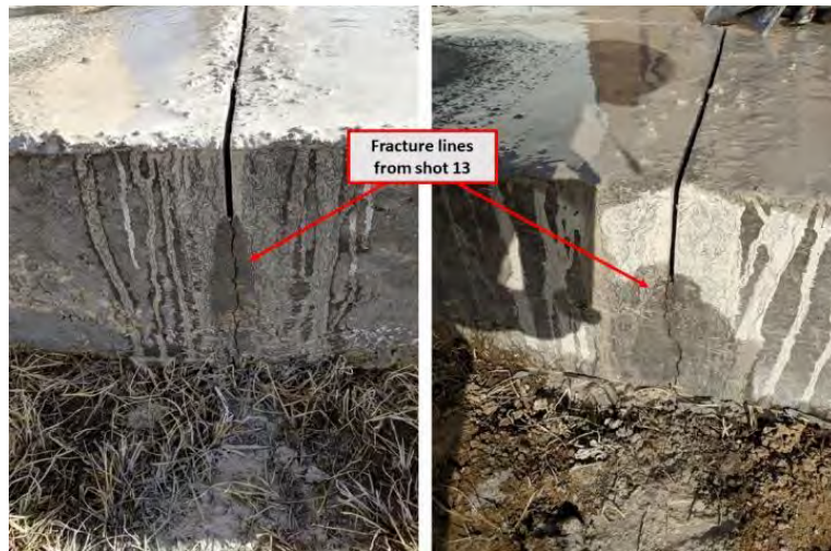
Figure 146. Shot 13: Fracture Lines from Borehole to Edge of Concrete Test Slab
