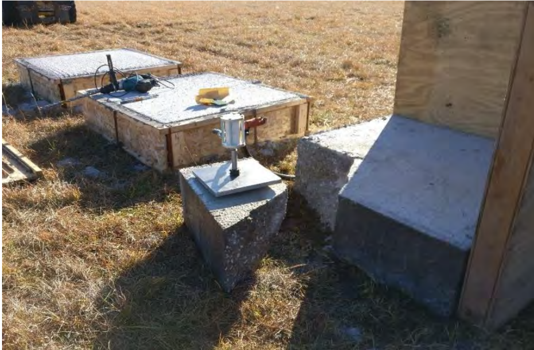
Figure 82. Shot 3: Plasma Blasting Probe Set up in Chunk of Concrete Separated by Shot 2
