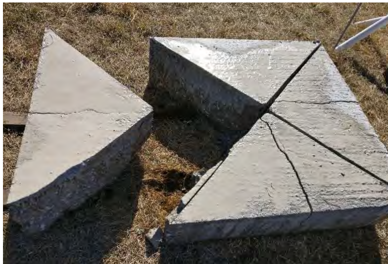
Figure 113. Shot 7: Test Concrete Slab 3 Section Separated by Shot along Pre-cut Lines
