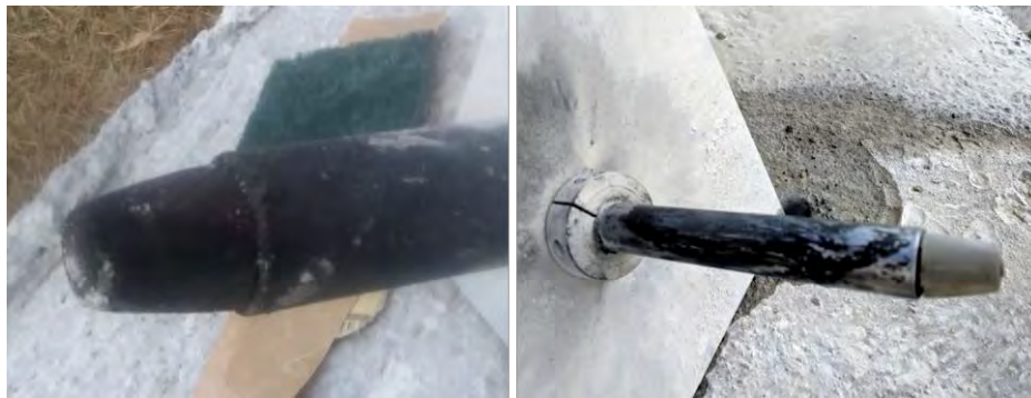
Figure 157. Shot 15: Plasma Blasting Probe after Dry Fire (Left) Probe Tip Is Slightly Bent, Significant Carbon Buildup. (Right) Cleaned Probe Shows Adhesive Delamination
