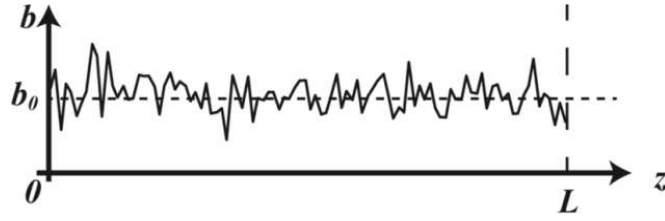
Figure 1: Example of random variation along tube axis; b is Pierce's detune parameter [4].
