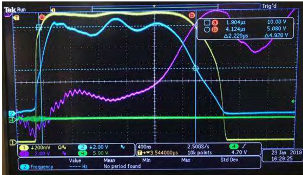
Figure 32: MG5193 magnetron under test at L-3 Communications. Ch1 (yellow) is the RF output signal. Ch2 (blue) is a Pearson current monitor with a rating of 0.1V/A. Ch3 (purple) is the voltage applied to the cathode. Ch4 (green) is a monitor on the thyatron trigger pulse. Maximum output RF power up to 2 MW was achieved for two magnetrons.
