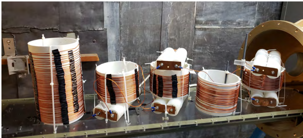
Figure 33: The eXtra Large Brass (XLB) pulse forming line, with capacitor pairs and air core inductors. Housed within a chamber provided by AFRL, the XLB PFN operates with an atmospheric pressure SF6 fill, producing 40kV for 3 \mu s into a 400 \Omega load.
