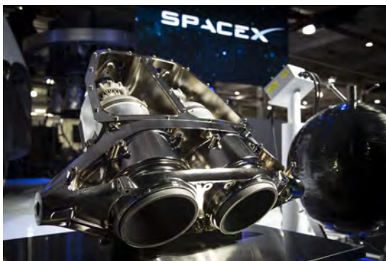
Figure H.3: SpaceX Super Draco Printed Thrust Chamber [454] (CREDIT: SpaceX)
