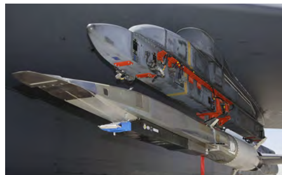
(b) X-51A Waverider on a B-52 (2010-2013 [359])
