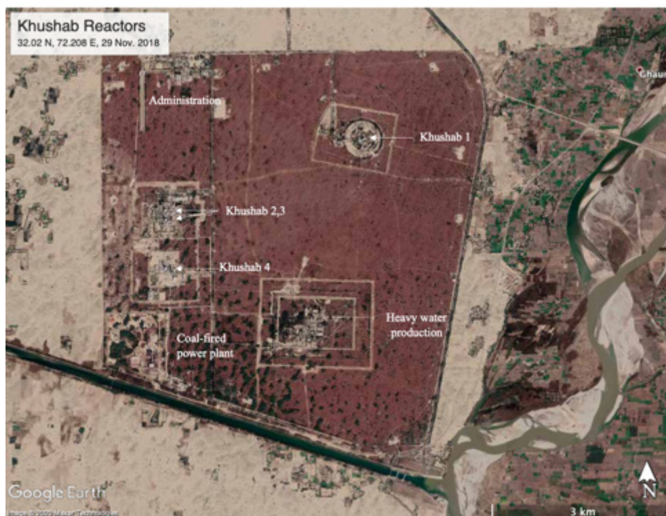
Figure 4.05: Each of Pakistan’s four plutonium-production-reactors and the associated heavy-water production plant has its own rectangular inner security perimeter within a single complex at the junction of a large canal carrying water from the Indus to the Jhelum River. The small bare areas just inside the perimeter fence of the complex appear to be anti-aircraft missile sites.
