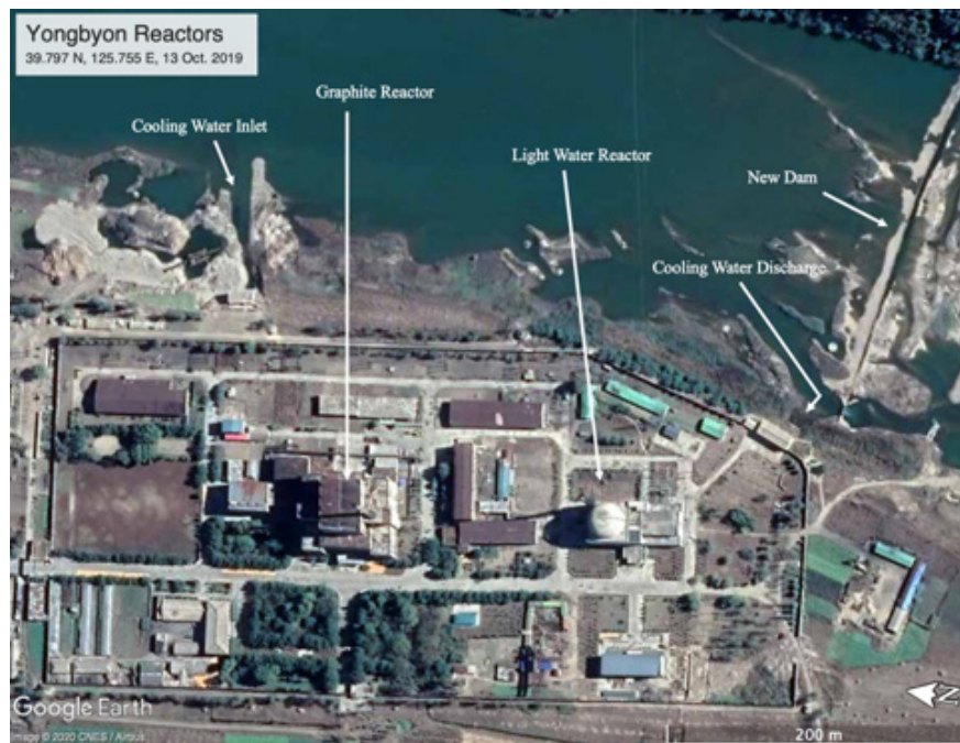
Figure 4.04: North Korea's two reactors in 2019. Left: the 20 MWt graphite-moderated, CO 2 -cooled reactor built in the 1980s based on the published design of the UK's plutonium-production reactors. Right: the dome of the containment of the 100-MWt Experimental Light Water Reactor built starting in approximately 2010.
