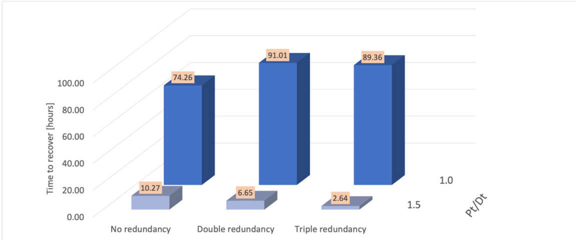
Figure 32. The sensitivity of time to recover to each microgrid ratio of power rating to demand and redundancy level.
