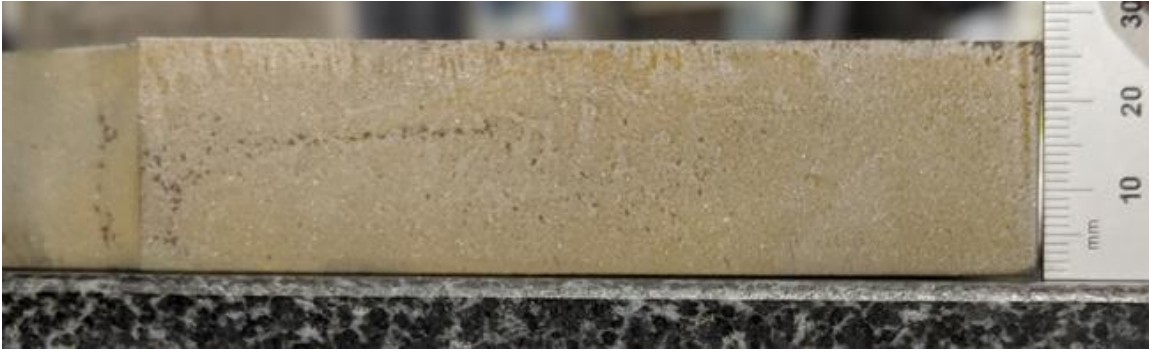
Figure 14. Image of the slight curvature (less than 1 mm [0.04-in.]) found in dog-bone shape portion of Specimen #3 post-welding.
