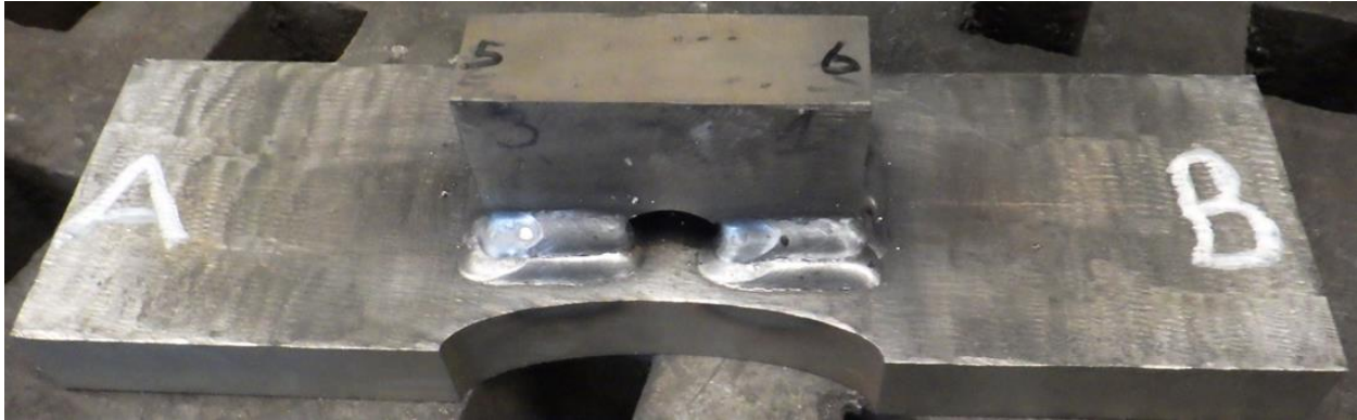
Figure 3. Post-welding to produce the final component, Specimen #3.
