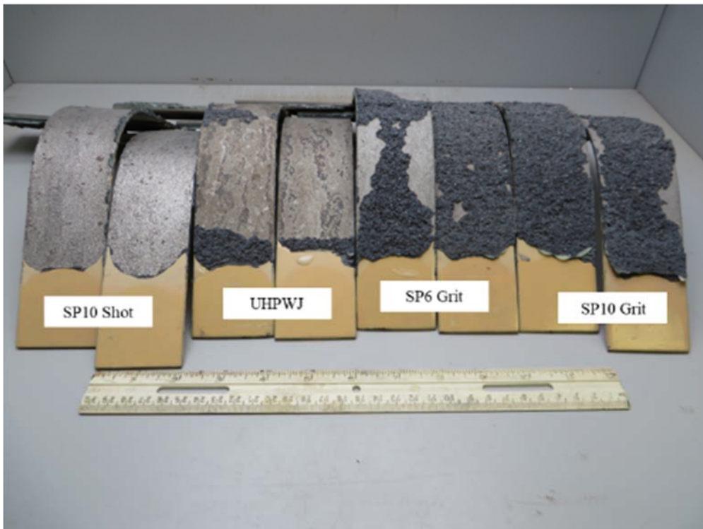
Figure 24 – Peel resistance results for Nonskid D
