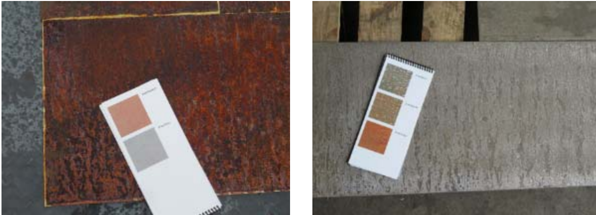
Figure 2 – Test panel after salt spray (left) and after UHPWJ (right) to remove rust and chlorides
