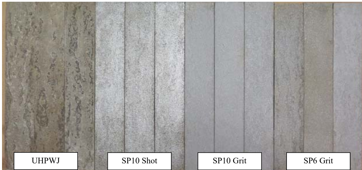
Figure 3 – Images of final surface preparation for test panels
