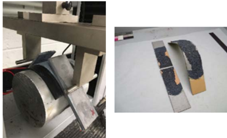
Figure 9 – Peel resistance test setup (left) and test panel after the mandrel bend (right)
