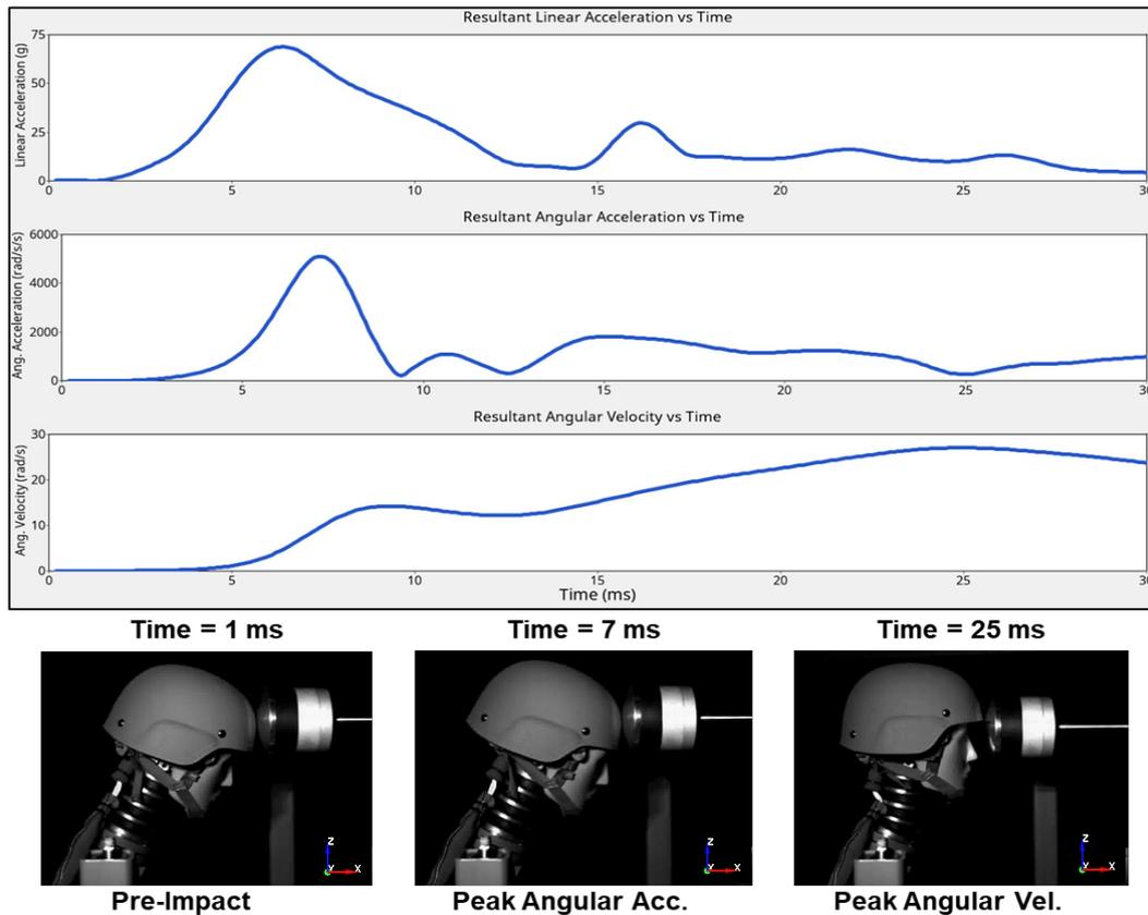
**Fig. 4** Example of resultant data traces for a pneumatic ram impact to the front of a Hybrid III head with ACH helmet at 14 fps. (Bottom) Images of the head and helmet at stages between pre-impact and peak angular acceleration during pneumatic ram impact. Compression of the front pads can be observed as the space between the forehead and helmet shell decreases. At peak angular velocity, the head is rotating and neck is flexing away from the impactor.
