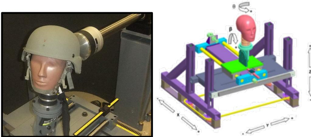
**Fig. 2 (Left) Pneumatic ram machine setup. (Right) Target assembly used in the pneumatic ram method consisting of surrogate head and neck on a translating table (Biocore 2019).**
