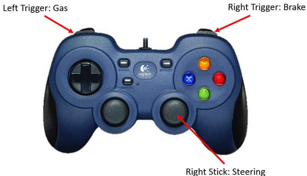
Fig. 2 Controller layout for robotic mobility operator's controls
