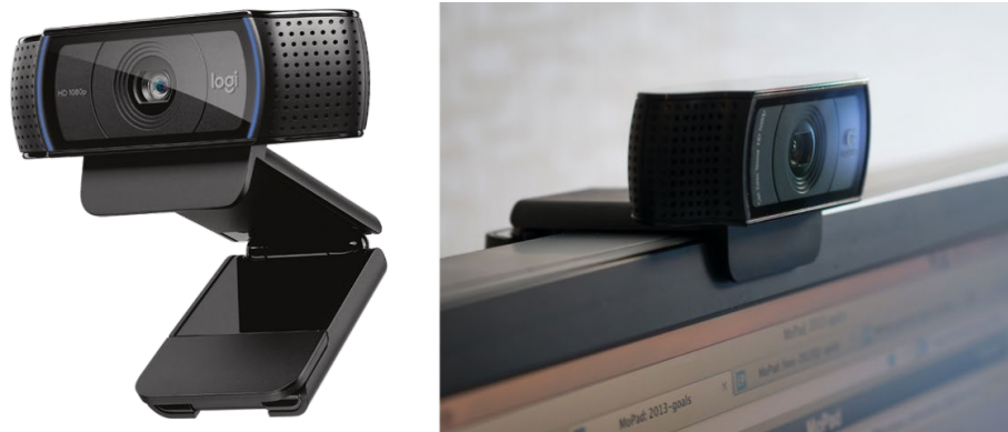
Fig. 5 Logitech C920 HD Pro Camera with autofocus and built-in stereo microphone; shown mounted on desktop monitor
