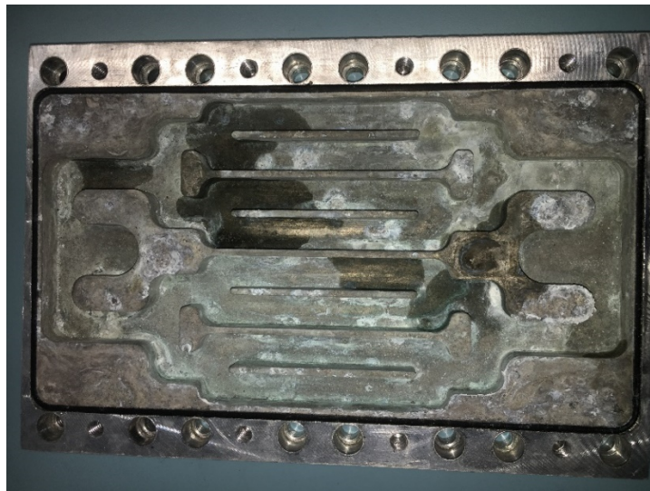
Figure 14. Water channels inside of the water cooler
