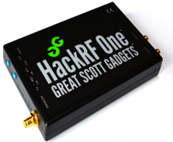
Figure 37. HackRF-One SDR. Source: Great Scott Gadgets (2016).
