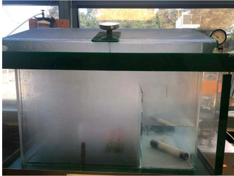
Figure 8. Salt Fog Chamber in Operation
