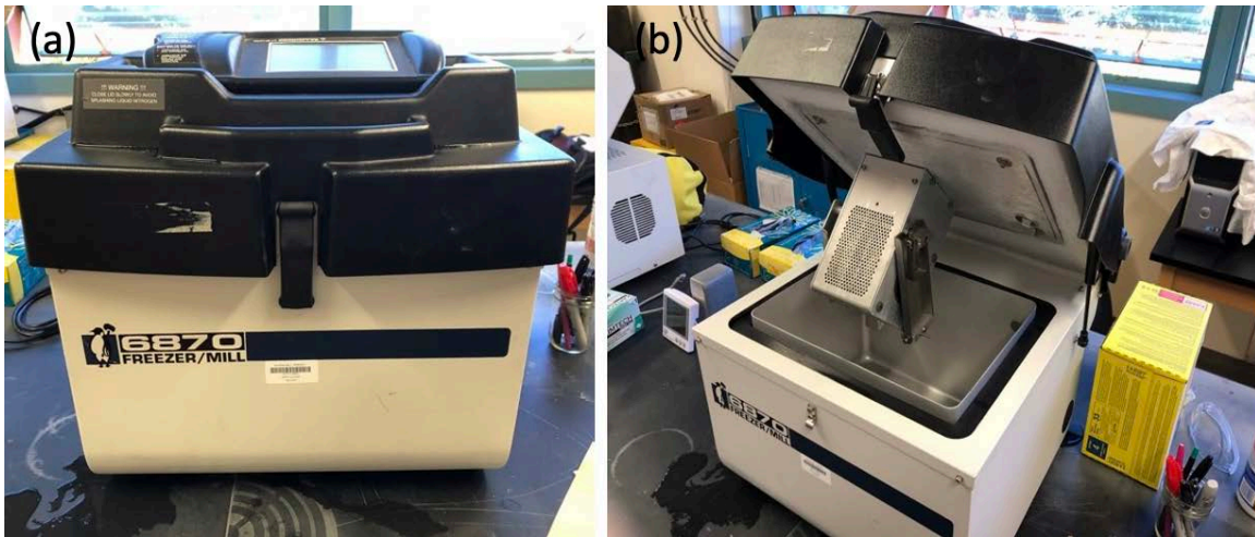
Figure 7. Spex 6870 Freezer/Mill Shown (a) Closed and (b) Open with No Liquid Nitrogen
