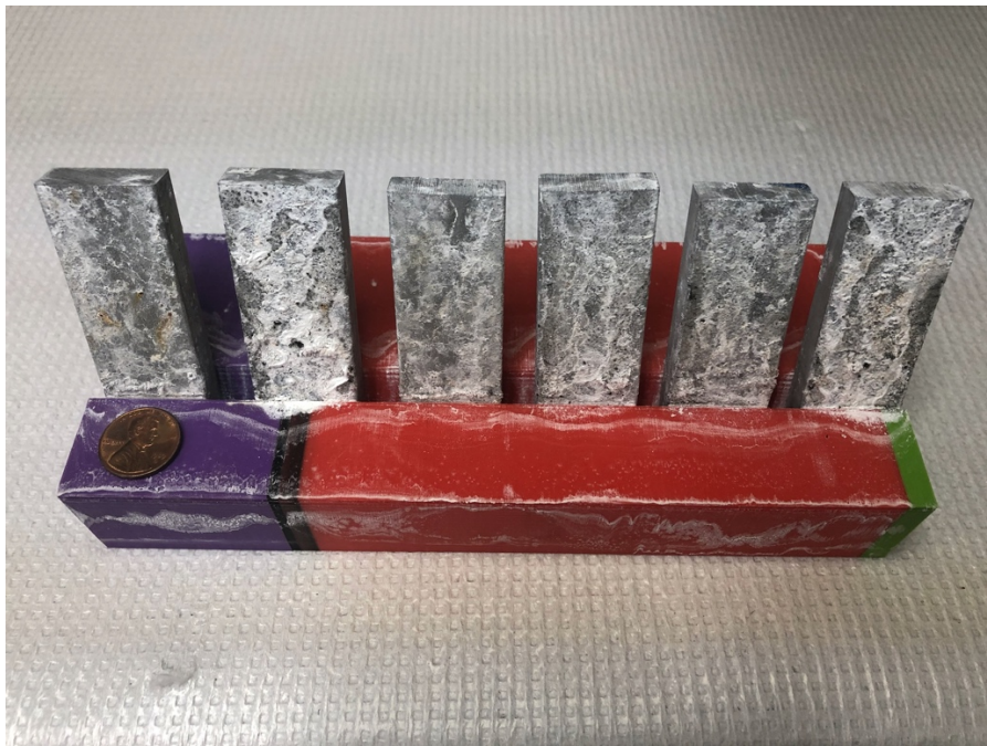
Figure 41. Sample Coatings in Order 1 Through 6, from Left to Right, Following 2000 Hours in a Salt Fog Chamber Accelerated Corrosion Test
