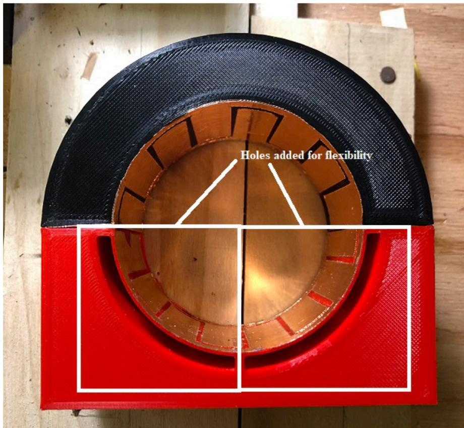
Figure 28. 3D printed assembly of final TENG design.
