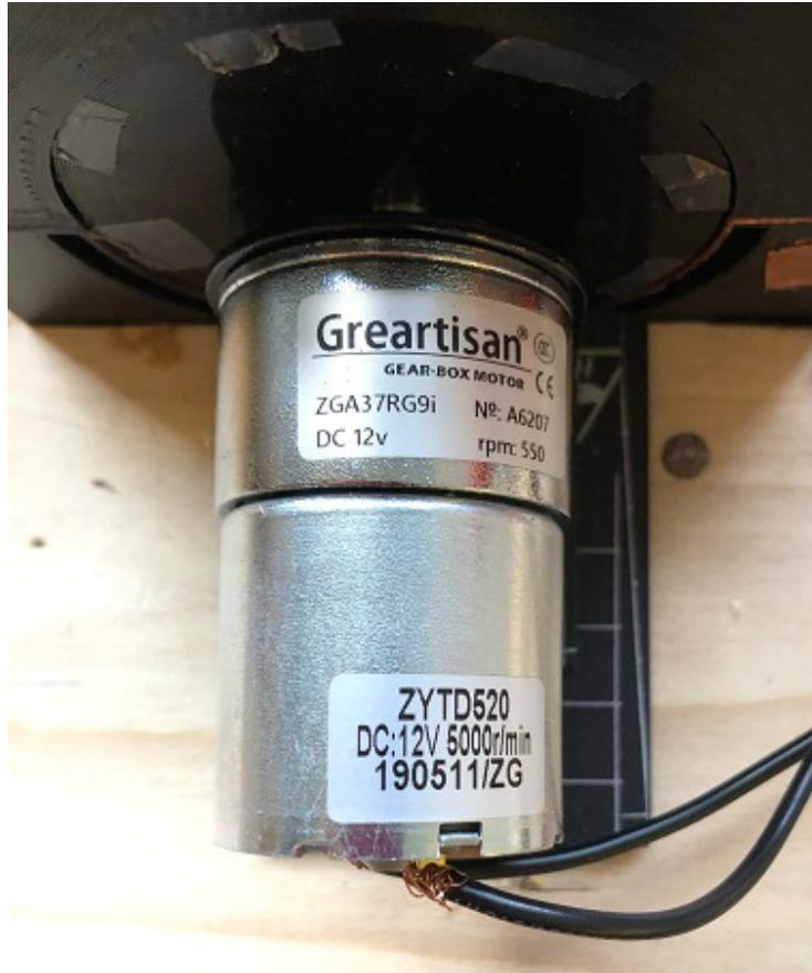
Figure 35. DC motor drives inner rod for TENG.
