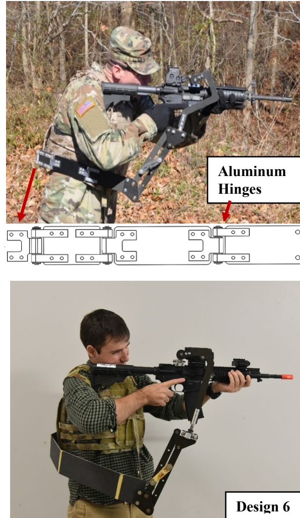
Fig. 17 Integration of multihinge composite panel into Third Arm
