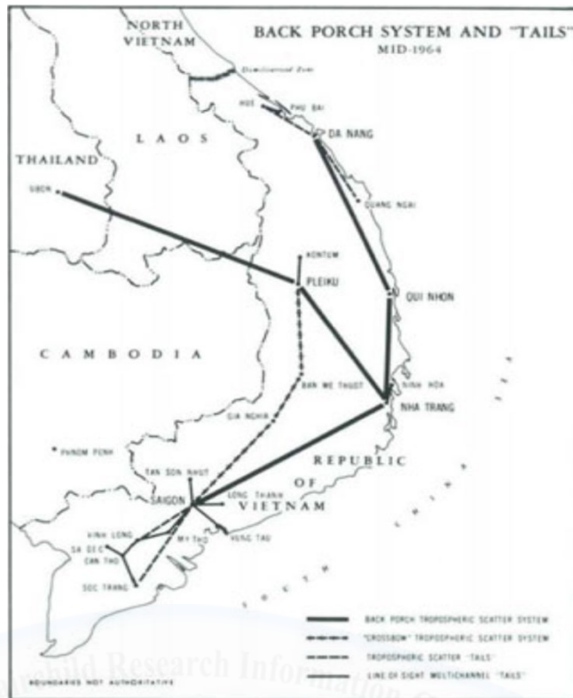
Figure 2. Back Porch System in 1964 (reprinted from Vietnam Studies: Communications-Electronics 1962-1970 )
