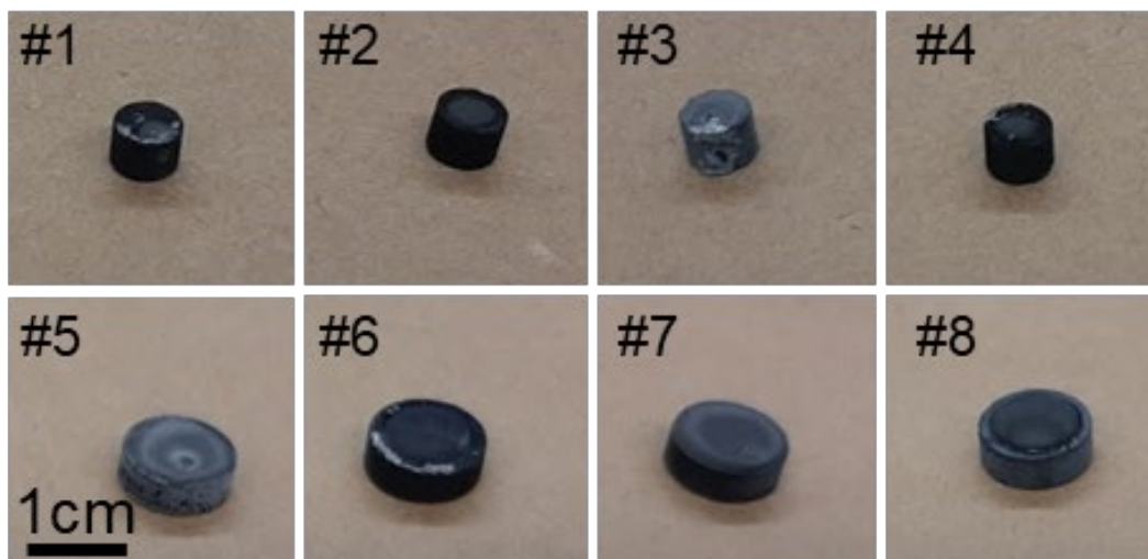
Fig. 22 AC DOE specimens from Table 7 after flash showing formation or absence of channels
