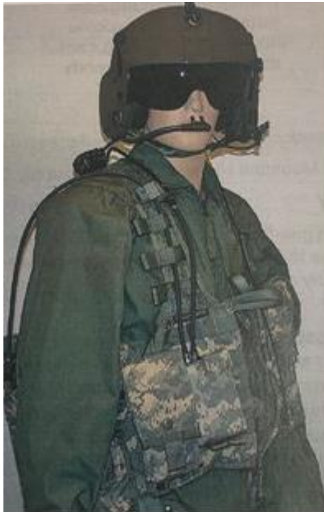
Figure 1. The PHODS mounted on a manikin illustrating its placement when in use.
