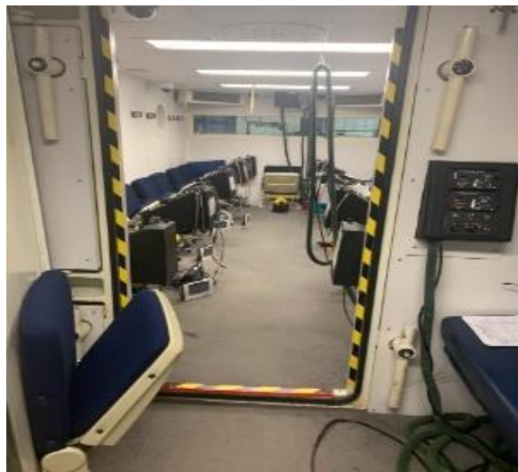
Figure 6. Inside view of the USASAM altitude chamber. Various test devices such as the Nonin Life Sense are visible on the floor of the left side of the chamber near the seats. With four evaluators, two USAARL TMs, and the USASAM observer, space was limited. The chamber operator and other research staff and observers were positioned on the outside of the windows visible at the far end of the chamber.
