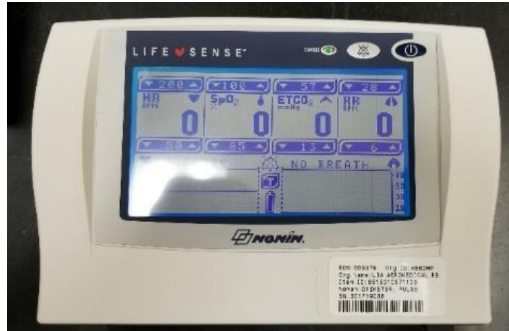
Figure 3. The NONIN Life Sense Model LS1-9R pulse oximeter monitor.
