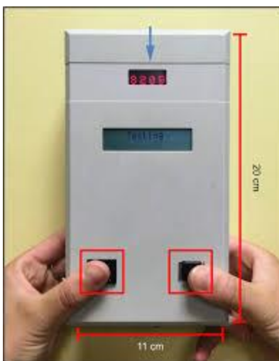
Figure 5. The handheld PVT-192 device. The blue downward pointing arrow at the top of the device indicates the window in which the red stimulus numbers appear.
