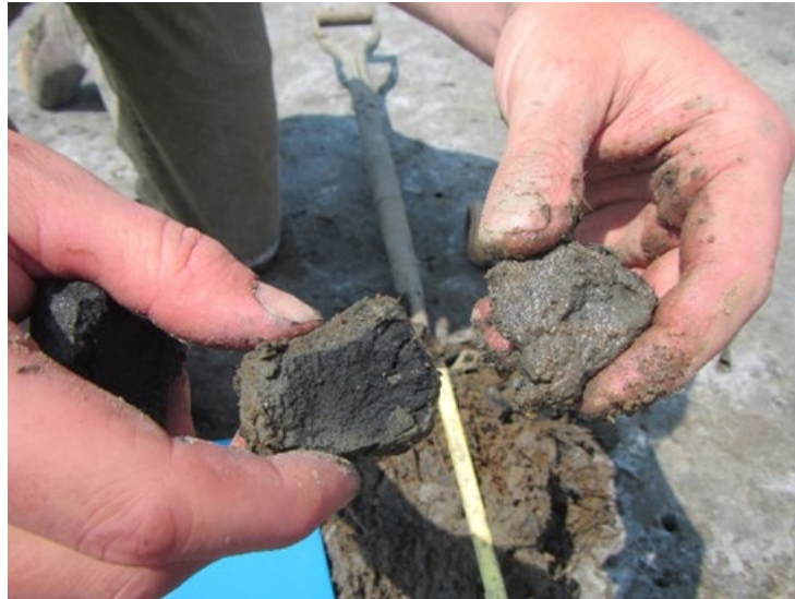
Figure 6. Dark soil coatings (soil on left) from acid sulfate soil materials at Avalon, then oxidized with 3% hydrogen peroxide (soil on right) resulting in removal of dark soil coating and revealing of the underlying grey soil matrix color.
