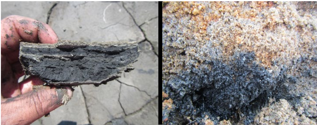
Figure 4. Avalon, New Jersey, soil sample (left) displaying extensive acid sulfate coatings with recently placed dredged materials; Narrow River, Rhode Island, soil sample (right) displaying black acid sulfate materials at the contact point between placed upland sands and the underlying marsh soils.
