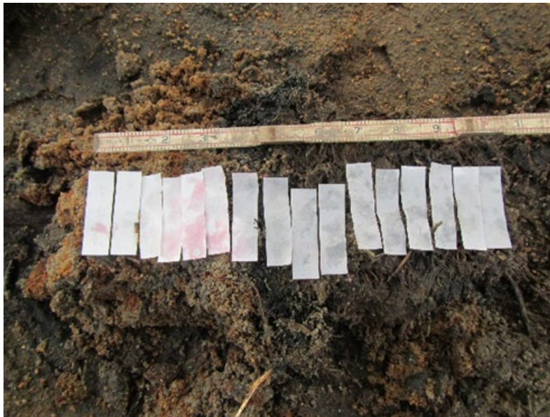
Figure 8. Reaction of reduced iron to \alpha -dipyridyl dye, seen as the development of a pink color, in the soil deposited on the marsh surface placed at Narrow River.
