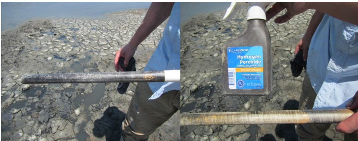
Figure 7. When present, free sulfides precipitate on the surface of IRIS tubes within one hour of installation, resulting in the formation of a black coating (left). Removal of black coating on the IRIS tube by hydrogen peroxide oxidation (right).
