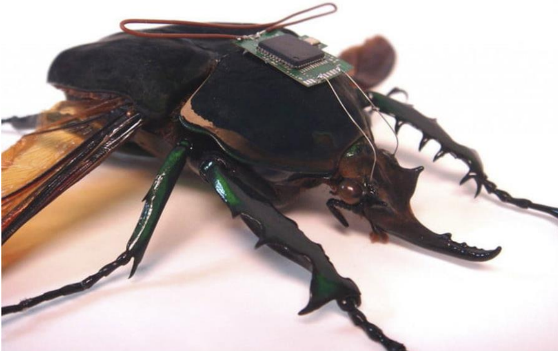
A cyborg beetle, part of DARPA's Micro Air Vehicles and Micro Electrical-Mechanical Systems research. DARPA has demonstrated ability to control insects in flight.
