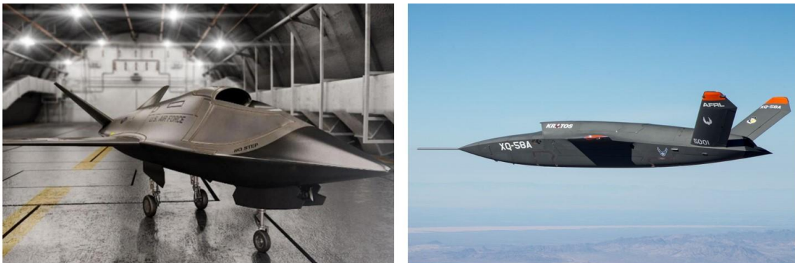
Pictures of the U.S. Air Force's XQ-58A Valkyrie, the robotic wingman for combat aircraft, first tested in 2019. It was designed with open-architecture, modular software, and hardware to enable 21 st century warfare in a way never considered.
