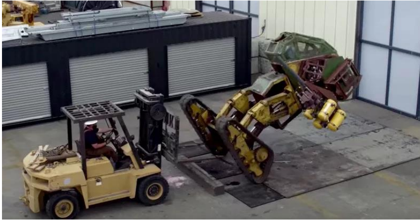
"MegaBots" tests the durability of its giant robot with a crash test. The top-heavy robot easily tips over. (Video screenshot by Bonnie Burton/CNET) Source: cnet.com
