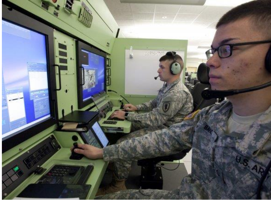
Figure 3. UMS pilot and payload operator interface includes large panel mounted display, joystick, keyboard, system switches and buttons, and center multifunction displays. (Source: https://www.army.mil/article/187989/army_simulator_provides_readiness_to_drone_flight_crews )
