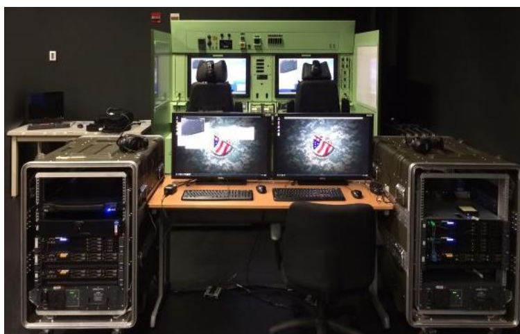
Figure 2. In the foreground is the operator's station. The green boxes are the computer system used to create and drive the simulation.
