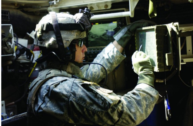
Fig. 4 Example of monitors in a combat vehicle (Center=CITV; Right=FBCB2; photo credit: US Army: https://www.army.mil/article/63135/army_links_tactical_radios_chat_services_with_commercial_communications )
