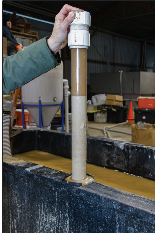
Figure 14. Recovered core used to compare against composited bed samples.
