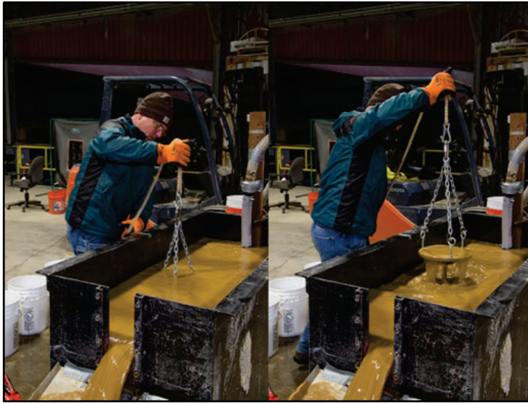
Figure 11. Deployment (left) and retrieval (right) of the plate sampler in the model hopper tank.
