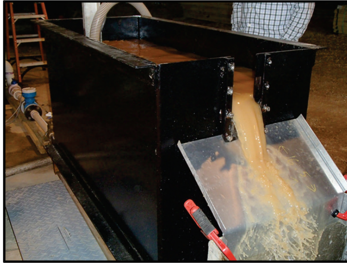
Figure 6. Model weir tank in overflow.
