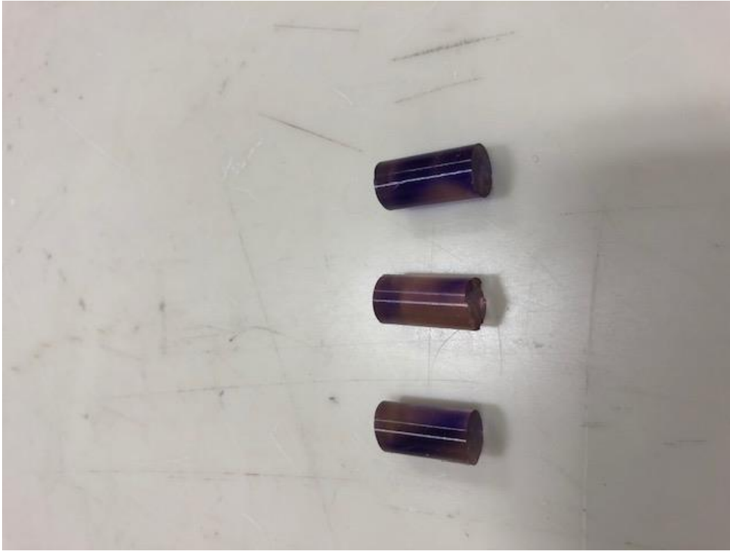
Fig. 9 Crown impact test (Experiment 1) posttest image of SP-PDMS
