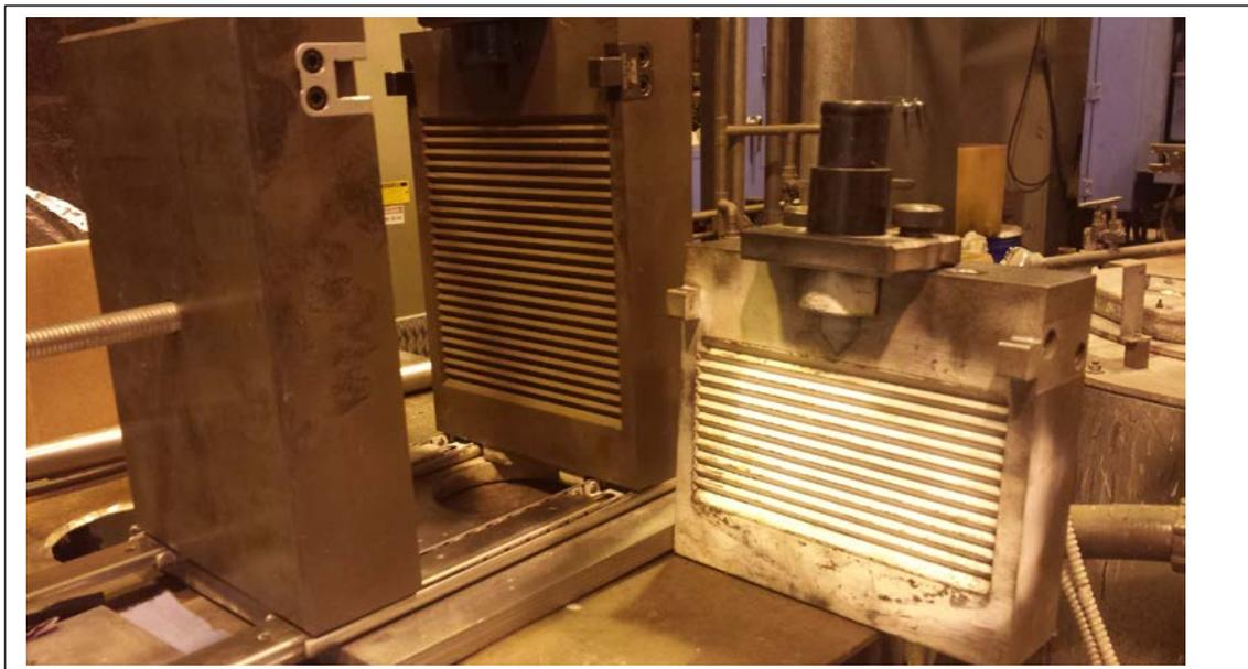
Figure 4.8: Installed large vent block side-by-side with old vent block
