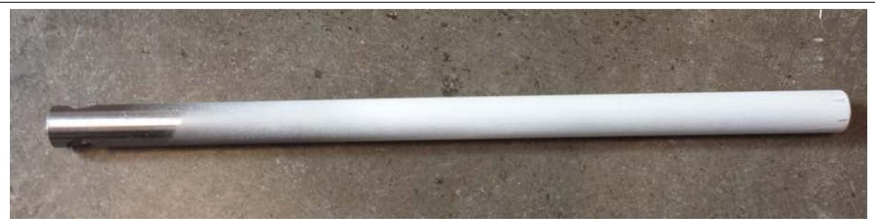
**Figure 5.4.2:** BN coated pull-out rod
