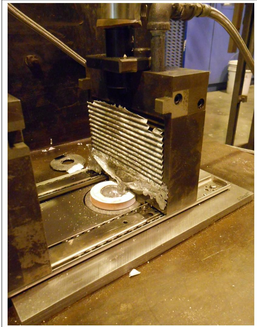
**Figure 4.6:** Open vent block demonstrating filling with aluminum
