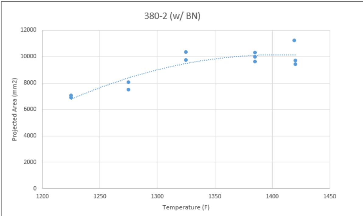
**Figure 5.2.11:** Fluidity of A380-2 using a BN-coated mold
