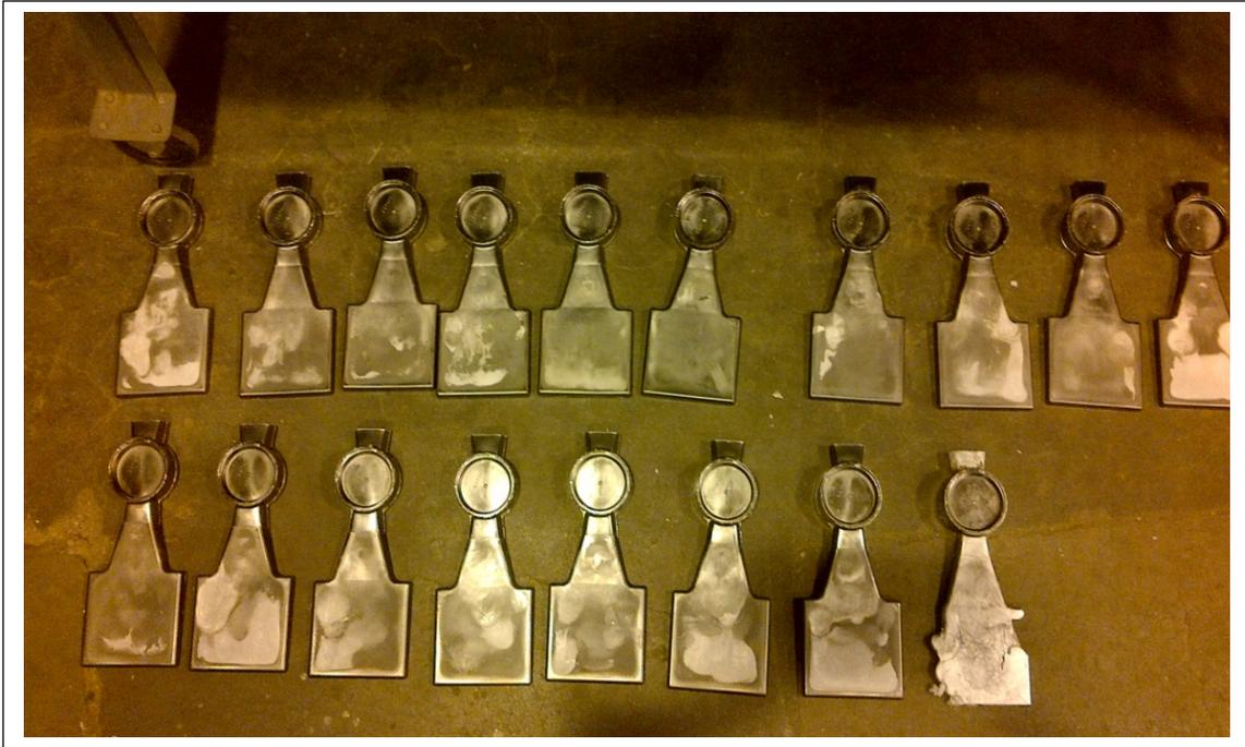
**Figure 6.4:** As squeezed cast 204 plates
