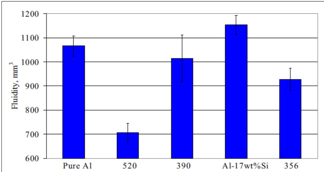
Figure 3.2.4: Relative fluidity of commercial foundry aluminum alloys
