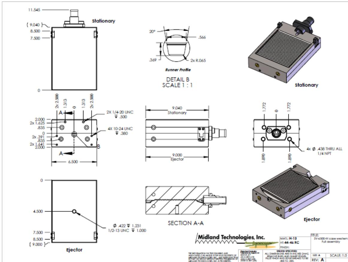
Figure 4.7: Schematics of the large vent block
