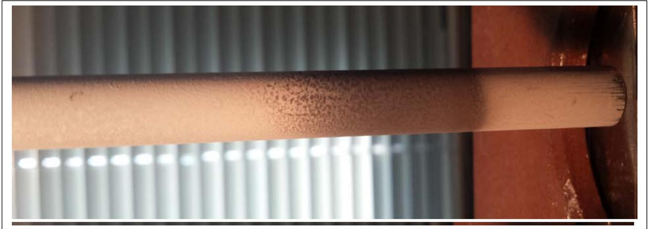
**Figure 5.4.5:** Smooth surface rod after first pull-out
