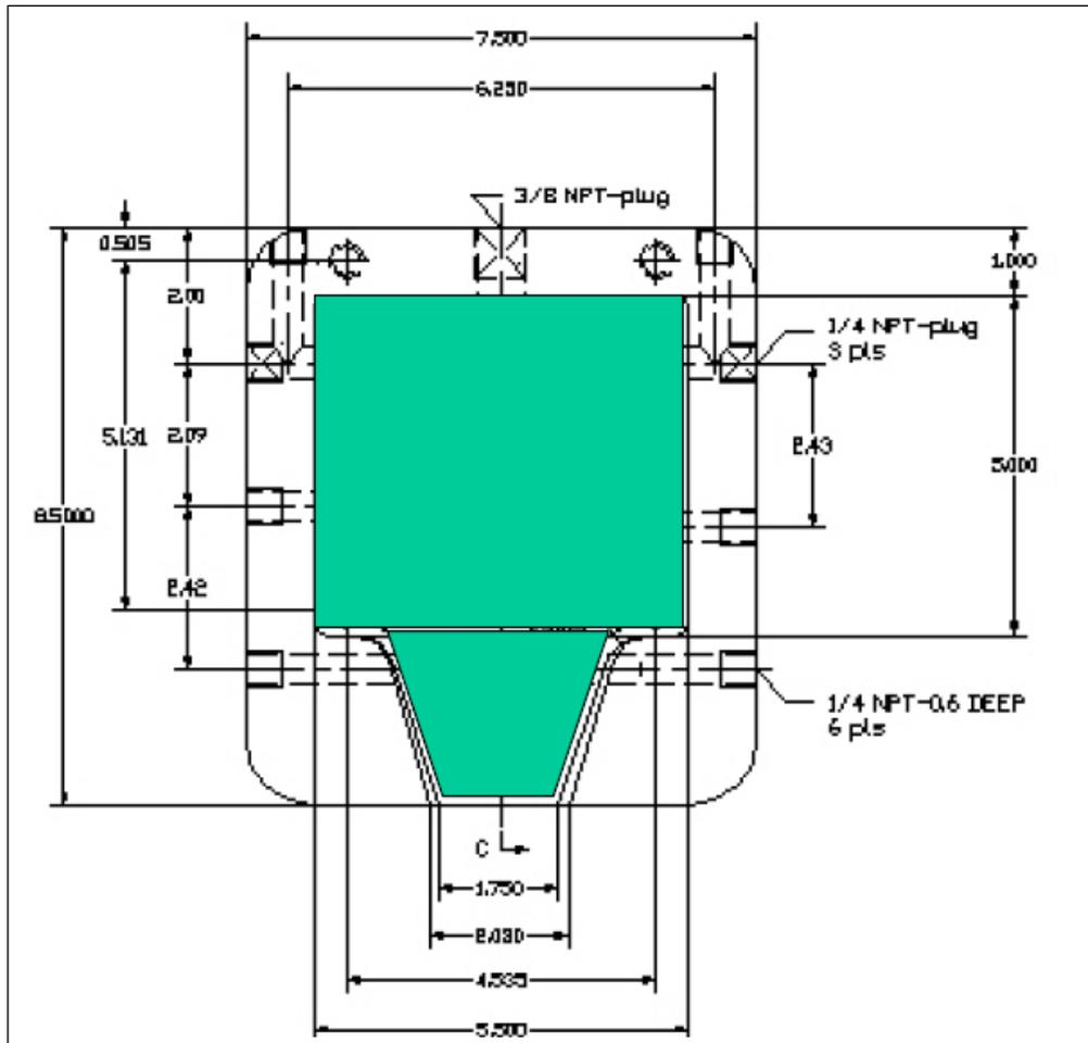
**Figure 6.3:** Squeeze cast plate dimensions
