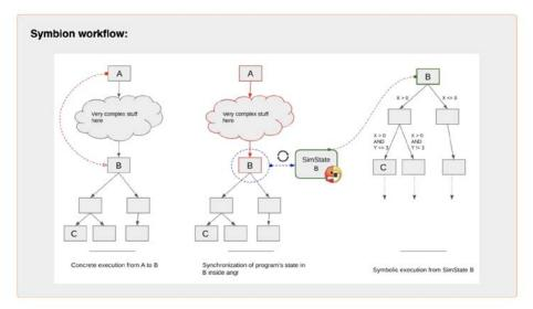
Figure 3-21: Overview of the Symbion path exploration technique [63]
