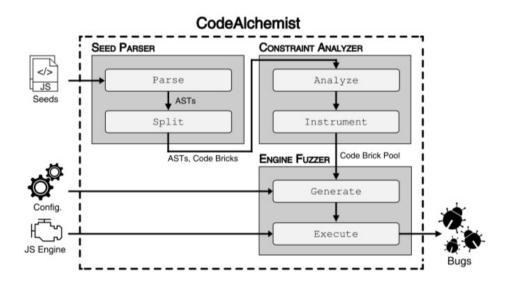
Figure 3-3: Architecture of CodeAlchemist [28, Fig. 5]
