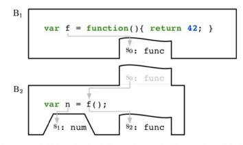
(b) Two code bricks obtained from the seed. The teeth and holes on each code brick represent the assembly constraints.
