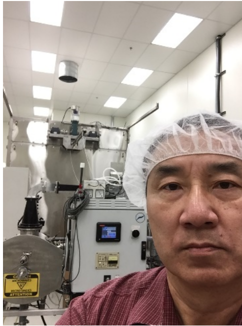
Figure 2. EnWave's 2 KW VMD system (E019; in the background of PI) uses rotation drum for drying
