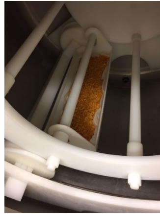
Figure 3a-c. a: 10-KW pilot scale VMD system (E040); b: Rotational drying drum; c: carousel drying trays
