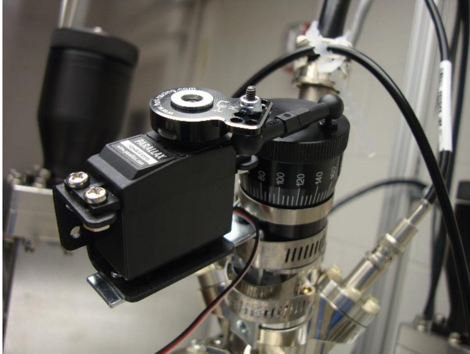
Figure 76: Actuator to rotate Faraday cup.
