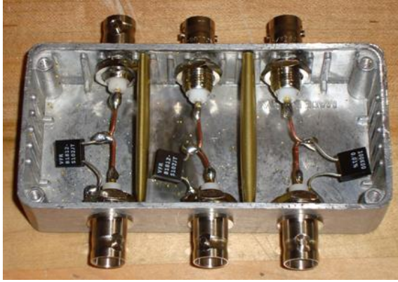
Figure 77: Low noise resistors (left); circuit model (right). Circuit model follows the conventional current standard.
