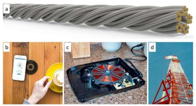
Figure 3. Litz wire and its uses. a, Schematic illustration of a hierarchically-twisted litz bundle of five bundles of five strands each (for 25 total wires). b-d, Example uses of litz wire at sub-MHz frequencies: b, Qi wireless charging mat. c, Induction stove. d, NIST WWVB timing signal transmitting tower.
