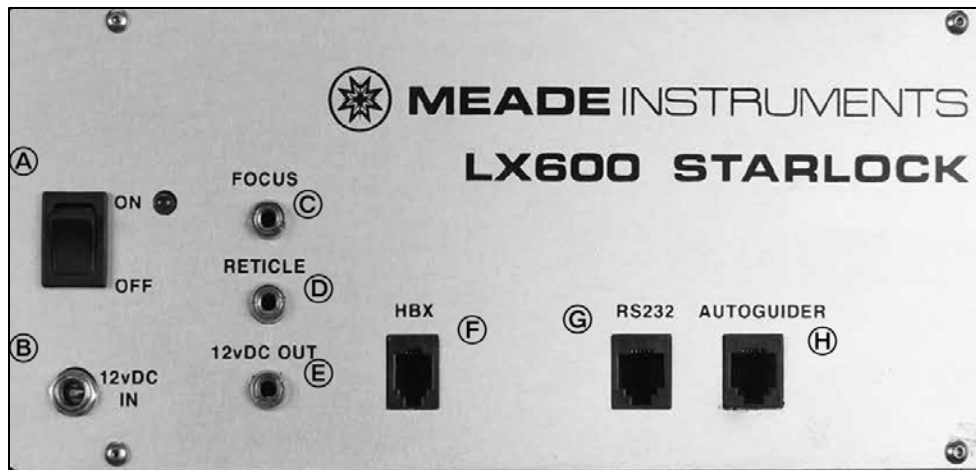
Figure 19. Meade LX600 Computerized Mount Interface. Source: Meade Instruments (2019).
