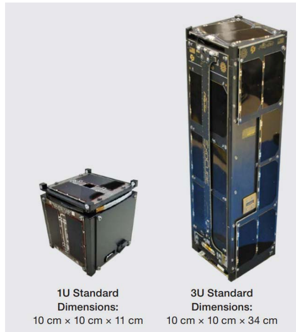
Figure 1. CubeSat Dimensions. Source: NASA (2017).
