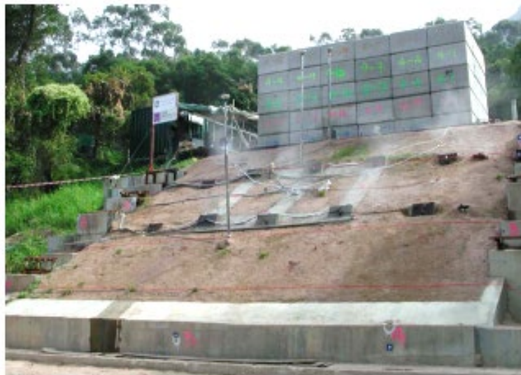
Figure 4. Loose fill slope testing with soil nails (Li et al. 2008).
