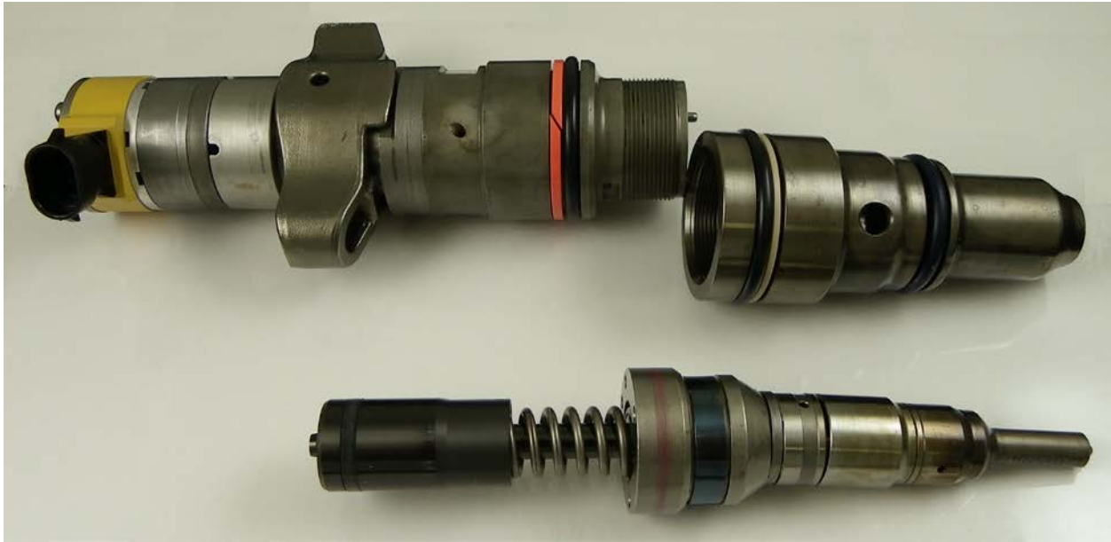
Figure 20. Caterpillar C7 HEUI Injector – Barrel Assembly Removal
