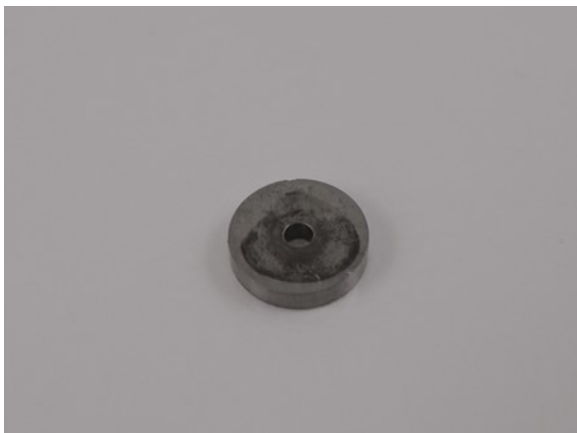
Stop Plate - Injector 3
