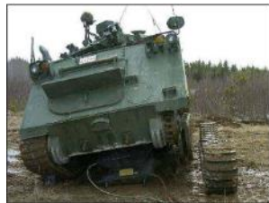
Band track difficult field repair
