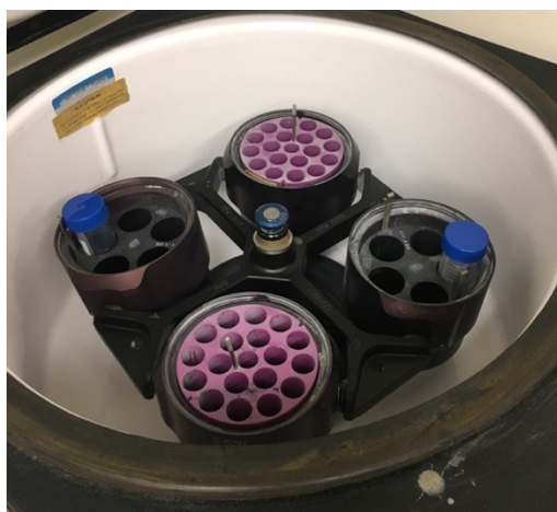
Figure 34. Centrifugal Separation of BNNTs
