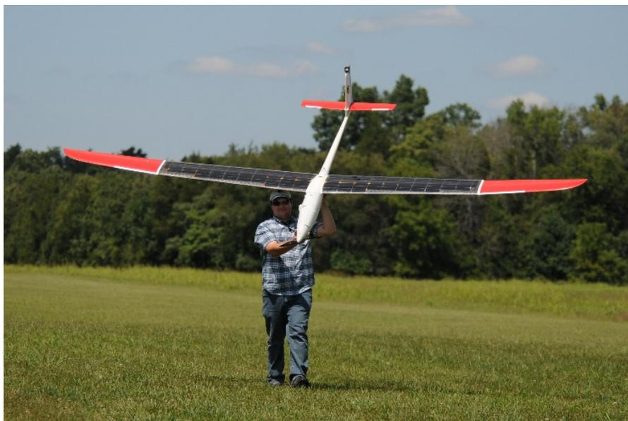
Fig. 3—NRL’s PV-SBXC UAV used for flight experiments
