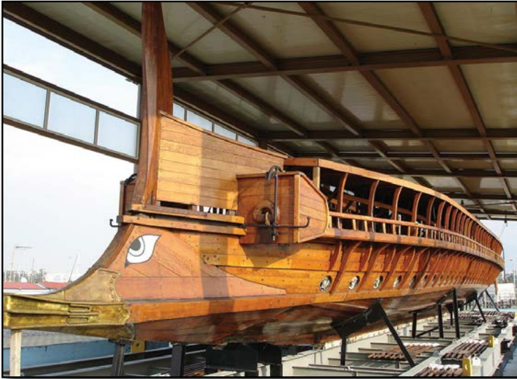
Olympias - A reconstruction of an ancient Athenian trireme with its ram. With trained oarsmen, the ram became an early and effective naval weapon.
