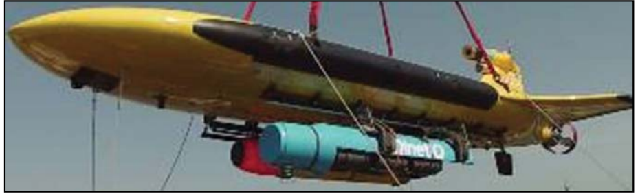
Manta Test Vehicle with Torpedo and Acoustic Sensors
