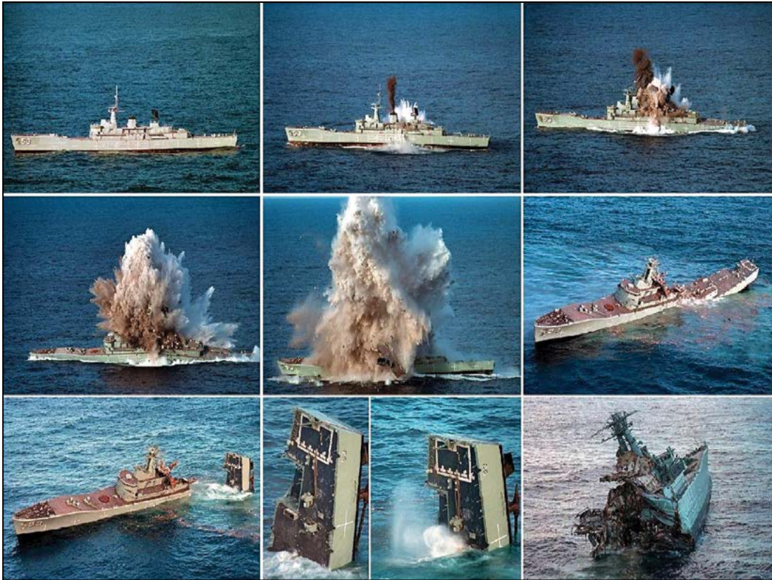
Sinking of the Royal Australian Navy Decommissioned River-Class Destroyer Escort HMAS Torrens by a MK 48 Torpedo Fired from HMAS Farncomb, a Collins-Class Submarine, in the Farncomb's Combat System Trials
