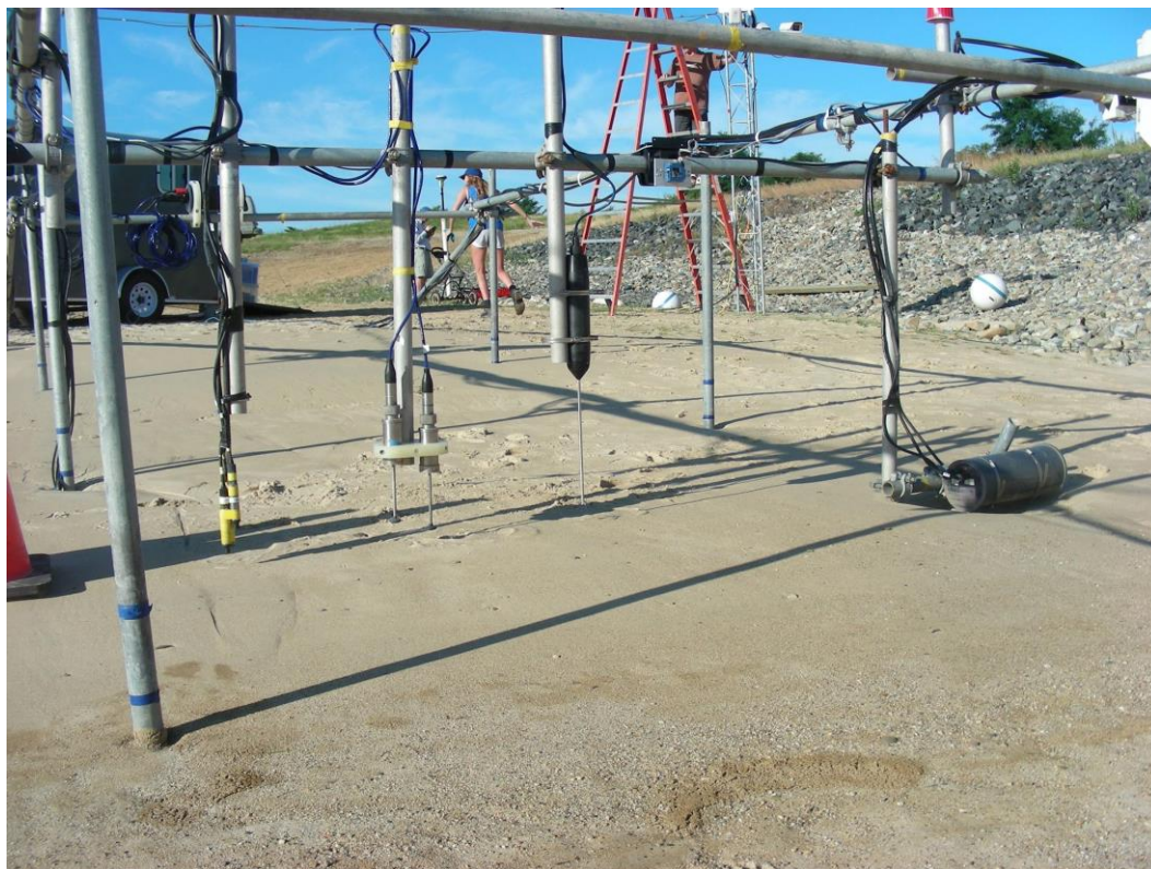
Figure 2. Picture showing field frame for deploying sensors. Sensors from left to right are: OBS array, EMCM pair, ADPV, Laser/Banner, underwater camera.
