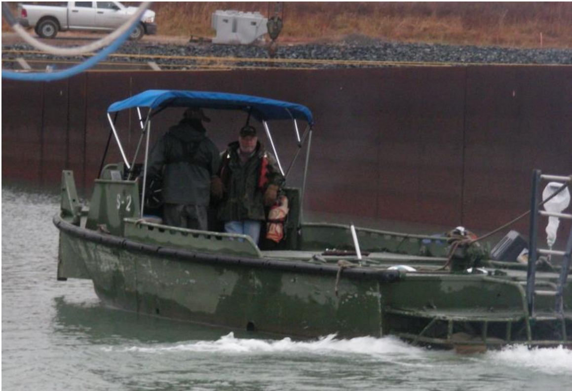
Figure 7. Picture showing vessel used for offshore surveys. The GPS antenna can be seen to the lower right (covered by a plastic bag due to rainy conditions). The sonar is located directly below the GPS.
