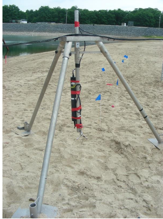
Figure 4. Picture showing tripod used to deploy Vector sensors offshore.
