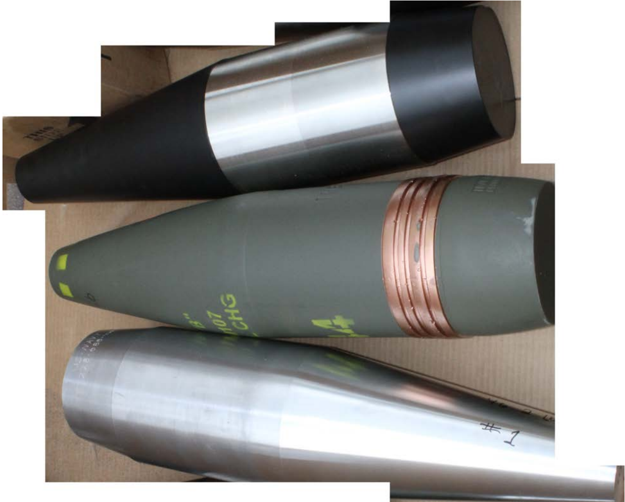
Figure 2. Photo of the surrogate (top), purchased replica (middle), and the replica fabricated from a single solid piece of aluminum (bottom) for the 155 mm, HE, M107 type. Note the purchased replica (middle) was determined to be positively buoyant and not deployed.
