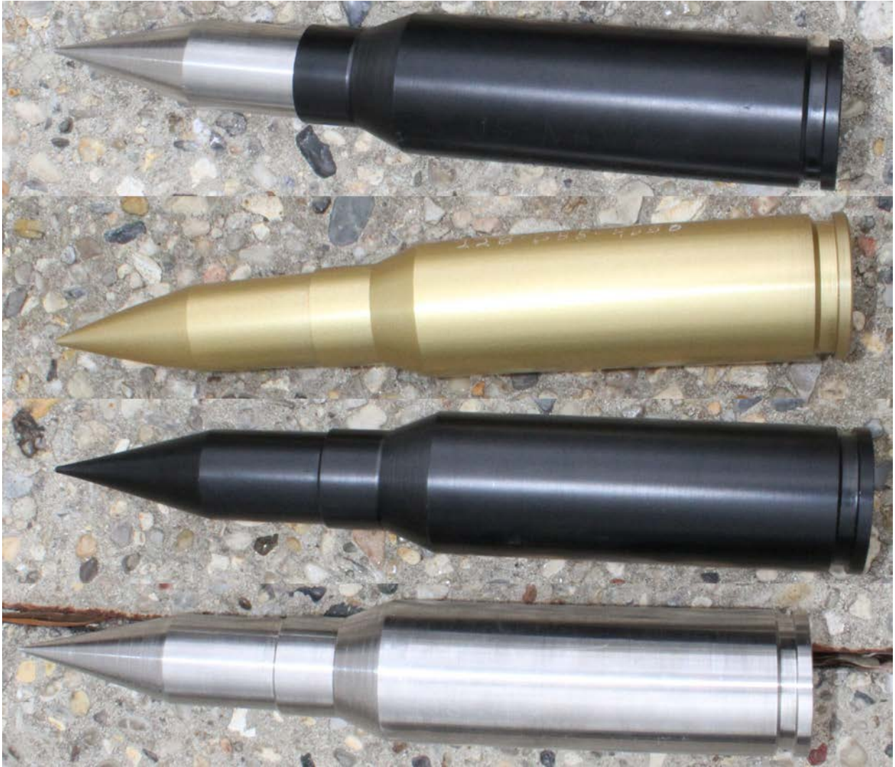
Figure 6. Photos of the surrogate (top), purchased replica (upper middle), the replica fabricated with solid Delrin (lower middle), and the replica fabricated with solid stainless steel (bottom) for the 25 mm cartridge type. Not shown was a similar set for the 20 mm type.
