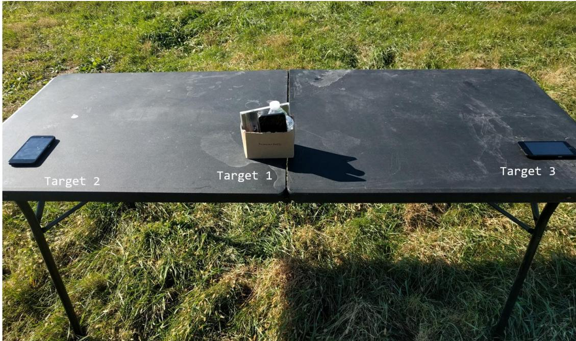
**Figure 32. Target orientations. Note each phone is oriented differently. Target 1 is propped up horizontally using a cardboard box. To prevent Target 1 from blowing away, a partially full water bottle is added to weigh it down while a Maroon 5 compact disk case kept the phone pointed toward the collection points.**
