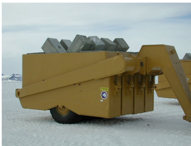
Figure 35. SW weight cart used for compaction on the roads and runways at McMurdo.
