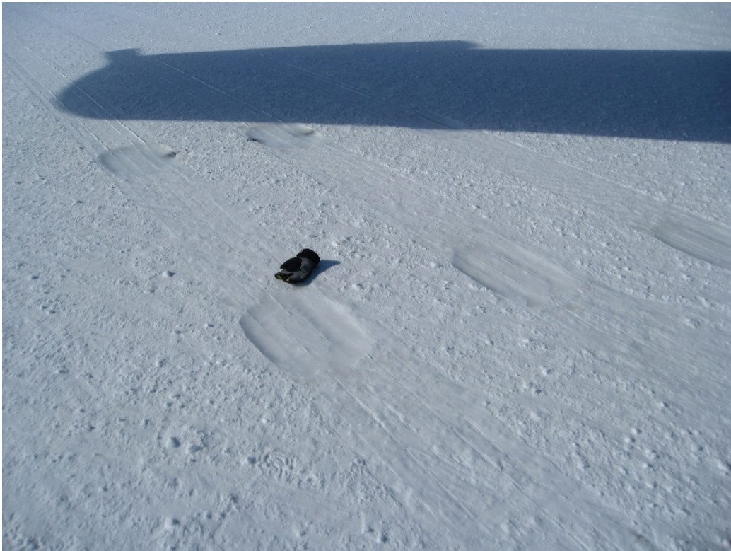
Figure 73. Snow creep depressions under each C-17 tire following approximately 40 minutes of parking time. The black glove in the picture is shown for scale.
