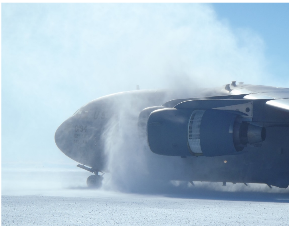
Figure 76. Snow whirlwinds forming in front of the jet engines during high reverse-throttle settings when attempting to back out of parking depressions.
