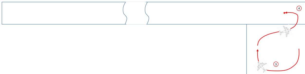
Figure 54. Push turn (4) to slide nose-gear tires on snow pavement.
