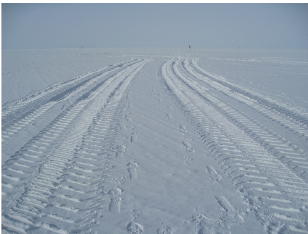
Figure 41. Parallel 50,800 kg (112,000 lb) compaction-roller tracks generated when moving from a very strong airfield apron (out of sight in the foreground) into a modestly compacted town site showing alignment of areas that supported the tire load (near-field tire tracks) and areas that suffered rutting (depressions further out).
