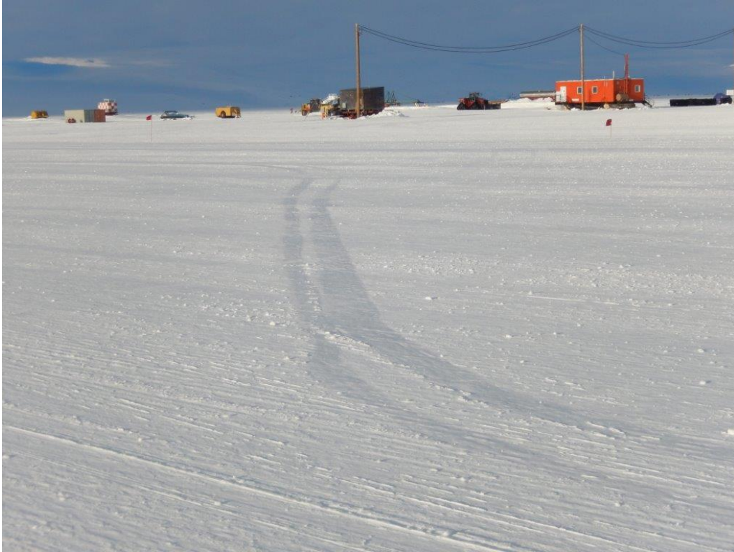
Figure 69. Tracks of the C-17's nose gear when "skidded" on the snow-pavement surface.
