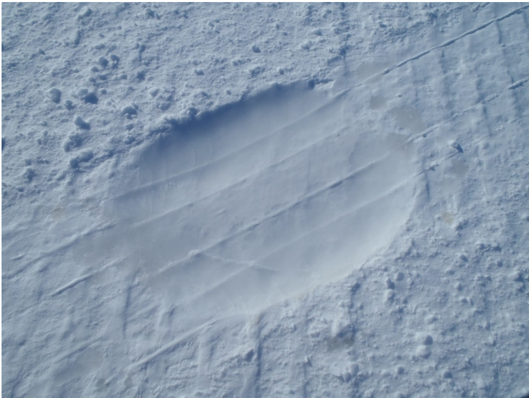
Figure 74. Thin melt-refreeze ice layer at the tire-ice interface of the parking depression.
