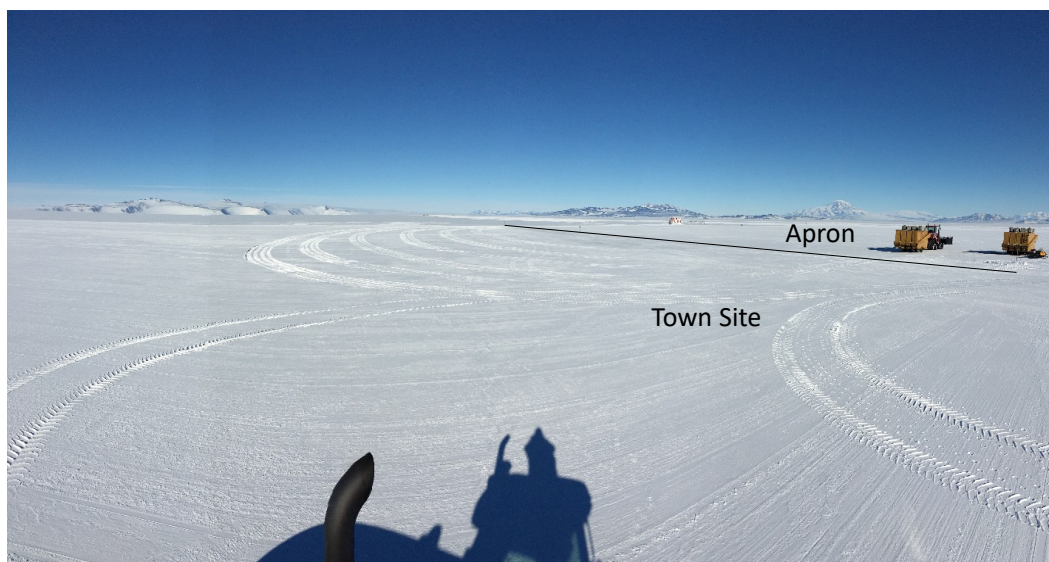
Figure 43. Arced paths of the 74,000 kg compaction roller traveling from the very strong airfield apron (in the background and to the right ) into the modestly compacted town site ( foreground and to the left ).
