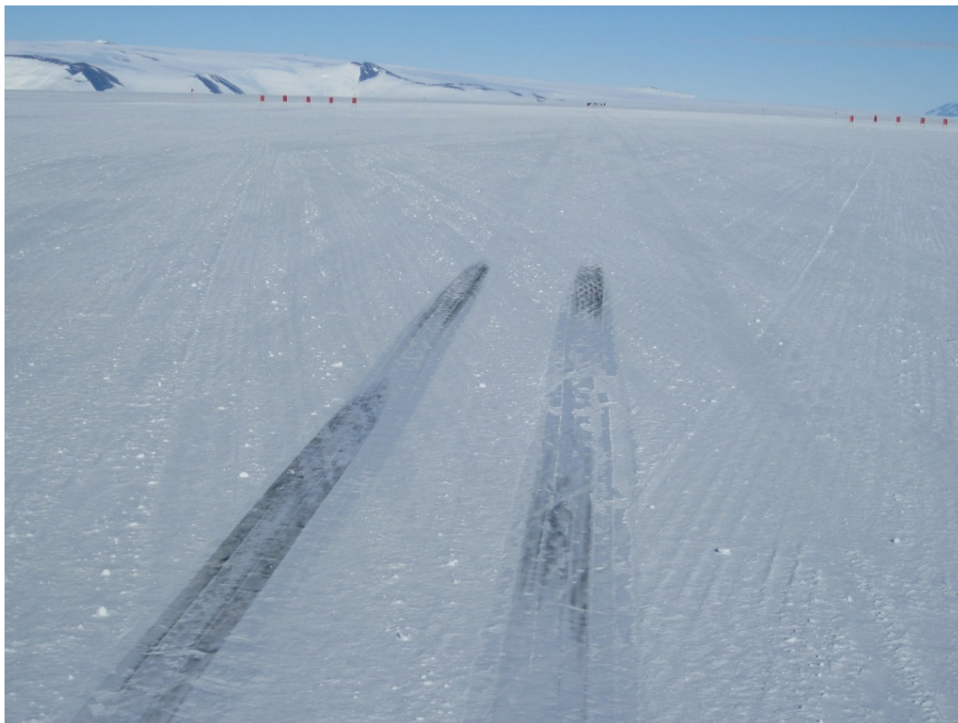
Figure 71. Tire rubber and a melt-refreeze ice layer associated with the main landing gear's spin-up during landing.
