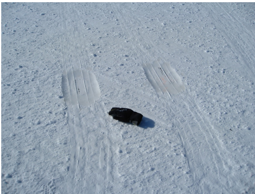
Figure 75. Depressions left in the snow by the nose gear during parking. The black glove in the picture is shown for scale.
