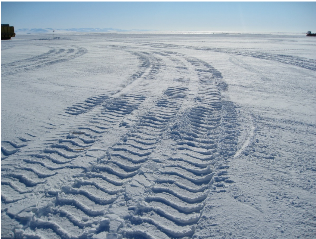
Figure 45. Compaction-roller tracks (movement in the direction from foreground to background) showing an area of Pavement Failure on the rightmost tire in an isolated region with the other tracks displaying only a Surface Disturbance response. Note the definitive difference between these two types of deformation where Pavement Failure displays disaggregation of the snow surface under the tire and “squeezing out” of this loose subsurface snow along the side of the tire.
