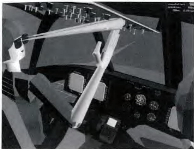
Figure VI-14. JACK. JACK, a 3D computer-aided design human figure model, is used to evaluate soldier interactions with weapon system design concepts.
