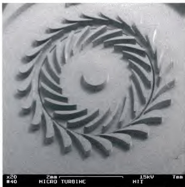
Figure V-10. Model Microturbine. Fabricated at MIT by ion-etching silicon. Diameter is approximately 2 mm. Research is part of the ARO program to power the Army After Next soldier.
