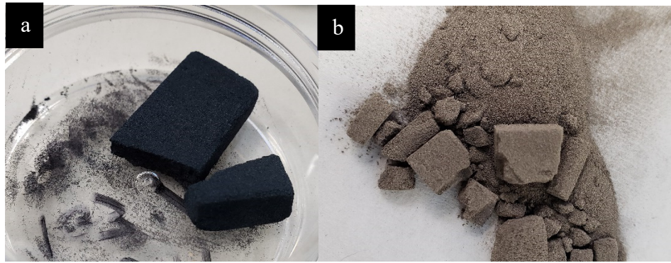
Figure 12. Sintered 3D-printed samples of H-10 aluminum. a) Sample 6 (760°C {1400°F} for 4 hours) b) Sample 2 (647°C {1196.6°F} for 8 hours)
