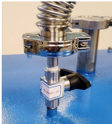
Figure 4: The TO PUMP/BURN OUT PORT VALVE on top of furnace
