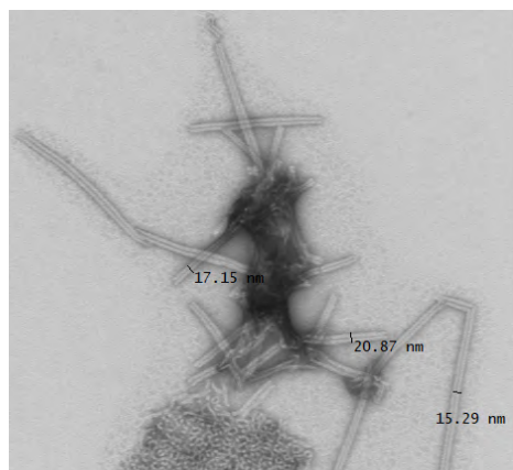
0.5 mM solution in 30% MeCN/water + 0.75% TFA heated at 60°C for 40 minutes, while constantly irradiated with visible light Visible light: 300 LEDs 12V, 72W
