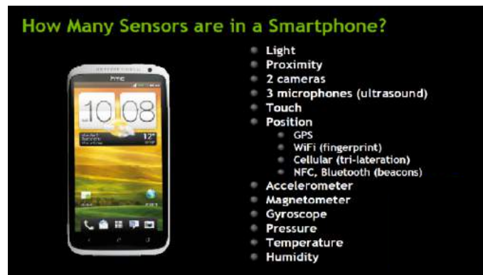
Figure 20 Sensors in a Typical Smartphone
