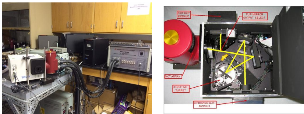
Figure 9: Picture of IR LIBS setup at HU employing an MCT array-spectrometer system (left). Close up picture of spectrometer with attached MCT array detector (right).
